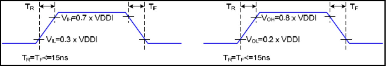
Figure 2 Rising and Falling Timing for I/O Signal
