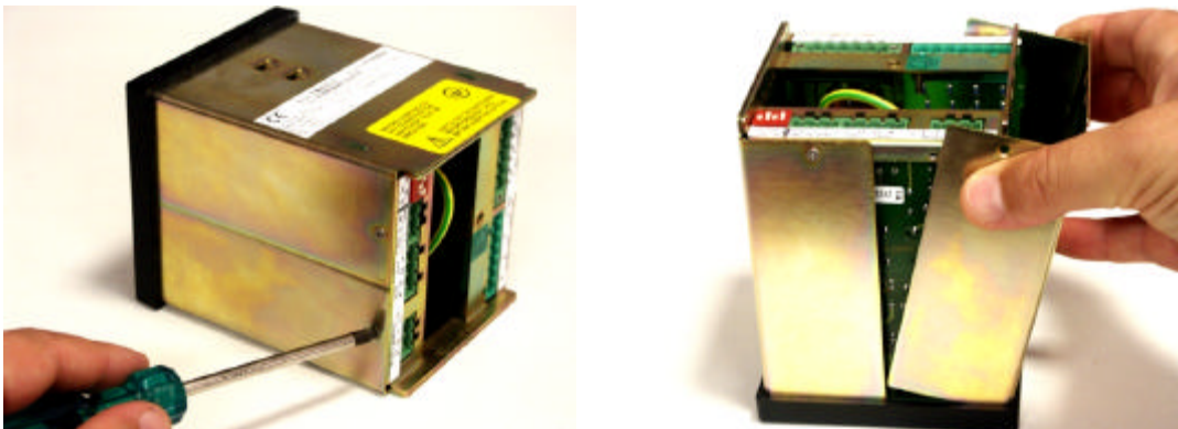
Pict. 4 – remove the bottom cover
