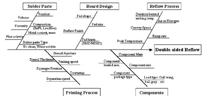
Fig. 4 Fish Bone Diagram for Second Side Reflow.
