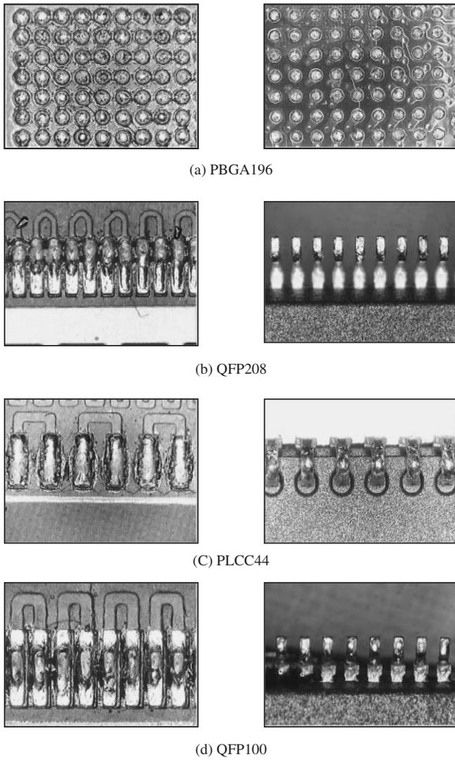
Fig. 13 Pads and Pin/Solder Balls After Components Fall Off.
