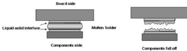
Fig. 3 Components Fall Off During the Second Side Reflow.
