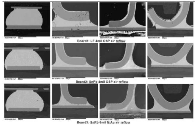
Fig. 14 SEM Pictures of Components Cross-sectioning.
