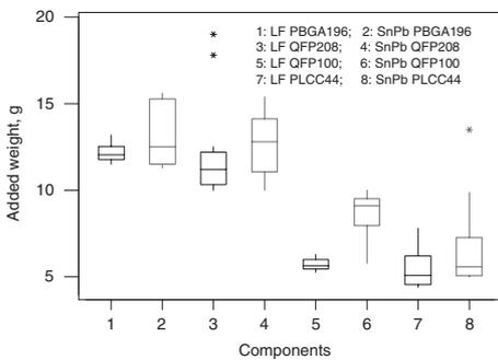
Fig. 9 Added Weight Comparison Between LF and SnPb.
