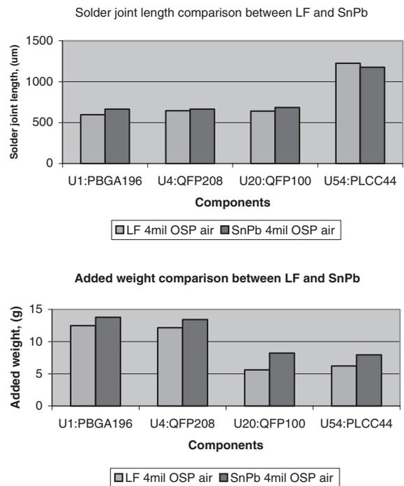
Fig. 15 Solder Joint Length and Added Weight Comparison Between SnPb and LF.
