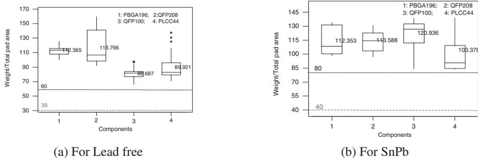
Fig. 12 The  $C_g/P_a$  Value for Different Components.
