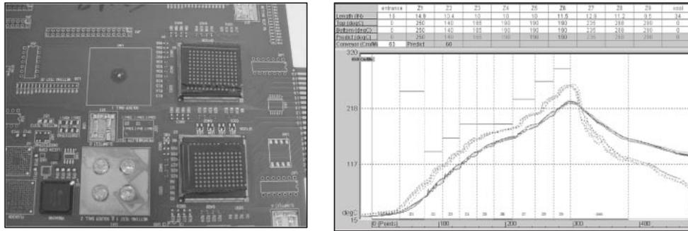
Fig. 7 PCB Weight and the Corresponding Profile with the Same Oven Settings.
