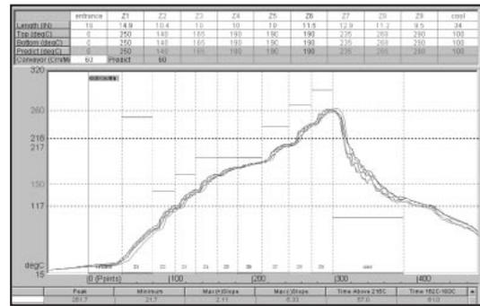
Fig. 5 Reflow Profile for Lead-free Assembly.
