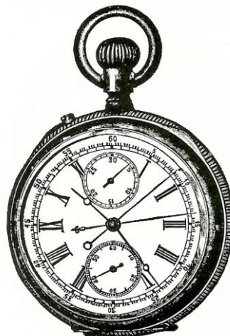
Guinand split seconds with minute register, extra glass cap, nickel movement, 13 jewels, Breguet hairspring, very reliable. No. 5865. Silver, engine turned case... ..$104 50 No. 5866. 10k gold, engine turned case... ..127 60 No. 5867. 14k gold, engine turned case... ..185 60 No. 5868. 14k gold, plain Boss case 197 20 No. 5869. 14k gold, border engraved box case... ..220 40 No. 5869½ 14k filled engine turned or plain case, 20 year guarantee... ..92 80
