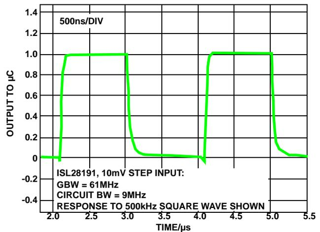
FIGURE 7. SIMULATED RESPONSE OF THE CIRCUIT IN FIGURE 5 TO A 10mV<sub>p-p</sub> SQUARE WAVE AT "Vc1". THE ISL28191 IS USED IN PLACE OF THE ISL28133
