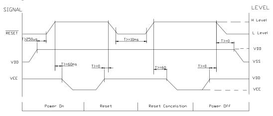
Please maintain the above sequence when turning on and off the power supply of the module. If VEE is supplied to the module while internal alternate signal for LCD driving (M) is unstable or RESET is active, DC component will be supplied to the LCD panel. This may cause damage to the LCD module.
