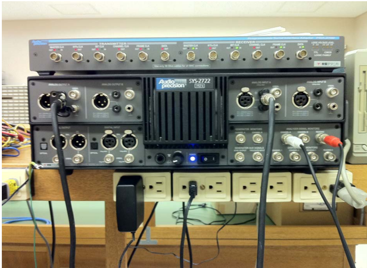
Figure 11 - The AP SYS2722 Distortion Analyzer Used to Characterize the Buffer
