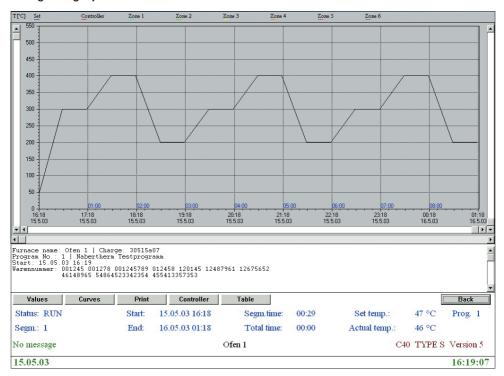
The upper part of the screen displays the programmed nominal value. Below information like furnace name, charge number, program number, start and end time as well as entered texts are displayed.
