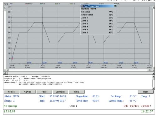
The visible area of the graphics can be moved with the grey scrollbar. With the white scrollbars the graphics can be zoomed, i.e. the temperature and time axis can be extended or compressed. This makes it possible to display an area of the curve in detail.
