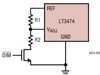
Figure 5. Dimming with an NFET and Resistor Divider
