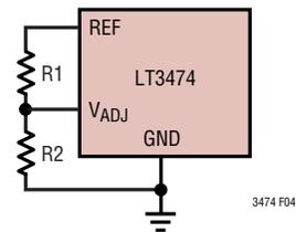
Figure 4. Setting V<sub>ADJ</sub> with a Resistor Divider
