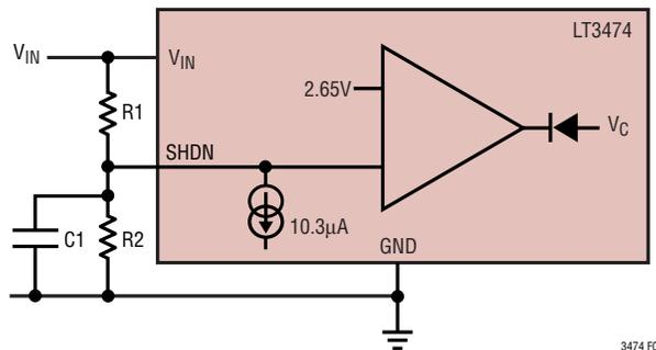
Figure 2. Undervoltage Lockout
