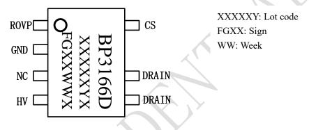
Figure 2. Pin configuration
