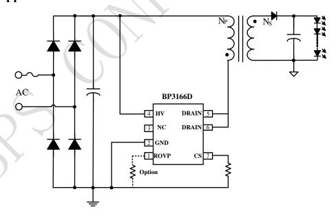
Figure 1. Typical application circuit for BP3166D
