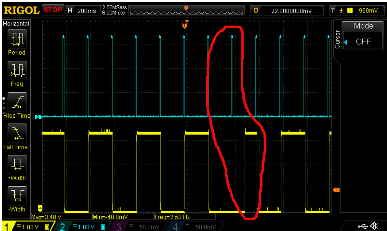
Illustration 2: Single Interrupts are not lost if hitting the device during ESP8266WiFiMult::run(). Blue channel interrupt input, yellow channel LED output)
