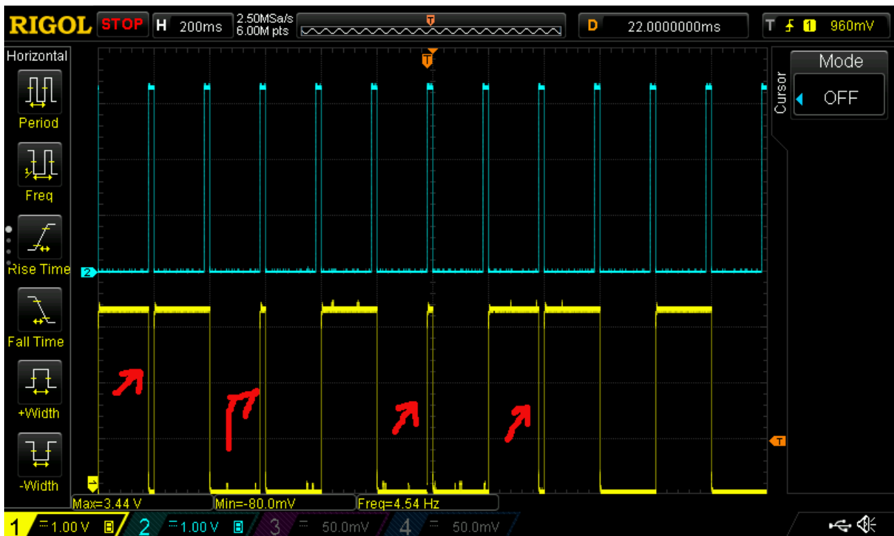
Illustration 3: Wrong generated Interrupts, generated not at falling edges. Blue: Interrupt input, Yellow: LED output
