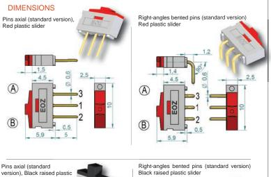
Right-angles bented pins (standard version) Black raised plastic slider
