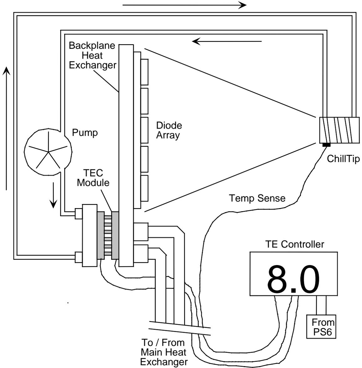
**Cooling Loop w/Standard Chill Tip™**
