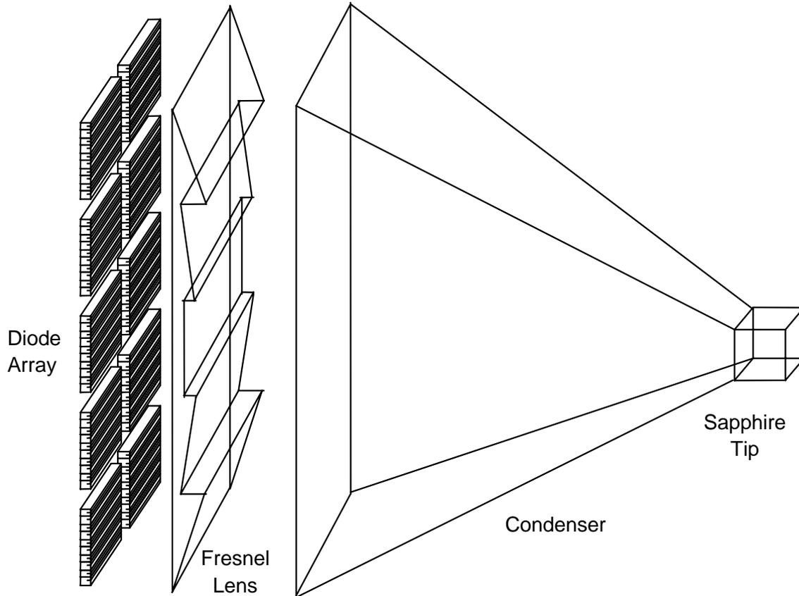
**Sapphire Tip (ChillTip™)** - the ChillTip™, a 9 mm x 9 mm square lens made of sapphire, is the output aperture of the Handpiece. Laser light is transmitted through the tip to the patient skin. To prevent tissue damage, the tip is wrapped in a cooling loop to maintain a tip temperature in the range of  $4 \pm 2$  degrees C.
