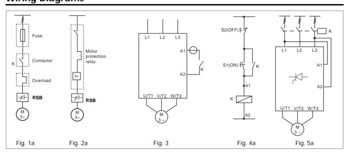
The motor controller provides by-passing of the semiconductors during running operation. Therefore the semiconductors can only be damaged by short-circuit currents during ramp-up and ramp-down. Please note that the motor controller does not insulate the motor from the mains.
