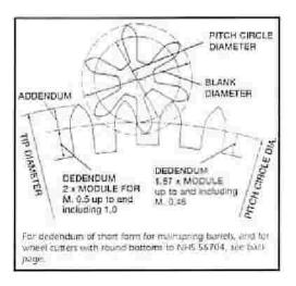
For cutting carbon steel pinions with high speed steel cutters
