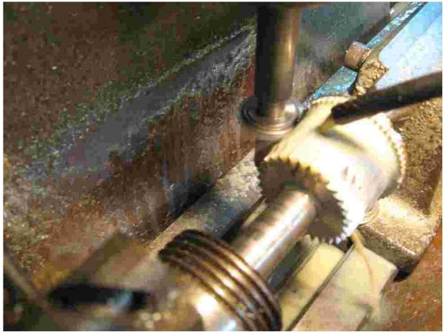
All Done! After shutting off the spindle the first thing I do is look at first tooth and last tooth to make certain I have not cut a 71 ½ tooth gear. Assuming all is well with the first tooth last tooth, I then measure the diameter of the wheel or pinion.
