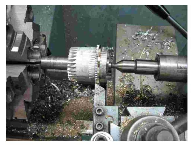
Here I am turning up the wheel blank on an arbor in an accurate 6 jaw and dead center. I leave the blank about .020" oversized and cut the teeth to the correct depth, then rebore the center holding the wheel by the tooth tips. This approach makes for an accurate sized wheel with no blunted tip teeth and a bore that is concentric with the teeth.
