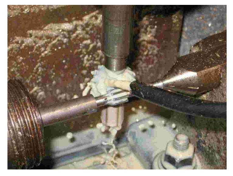
In cutting pinions coolant / lubrication is absolutely required. Cutting speed in this case is 255 rpm. You may be limited by spindle speeds but when cutting steel, too slow is better than too fast on speed of cut (feed) and speed of rotation of the cutter.
