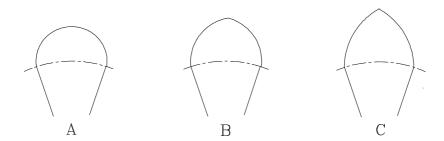
For driving gears, the wheels in a clock, the size and shape of the addendum are not arbitrary as the addendum is a working surface. The shape should be an epicycloid, but in practice a circular arc is used instead. The question facing horologists over the years has been how to choose a small standardised set of circular arcs to adequately approximate the infinite range of epicycloids required by the theory.
