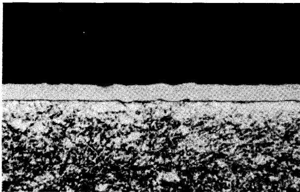
Figure 12. Nickel Plated Contact Fretted for 2 Hours at 200 gm. Original mag. 750X.
