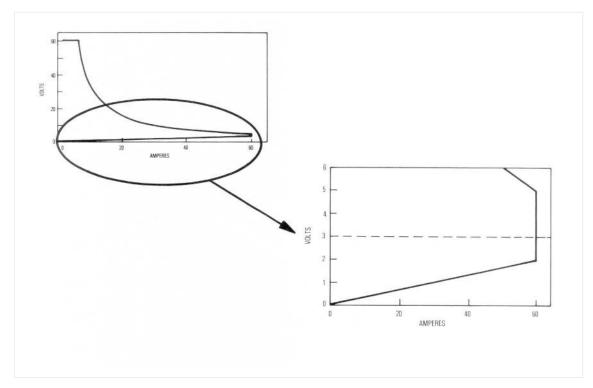
Figure 8. Operating Characteristics of a Keysight Electronic Load
