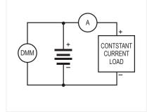
Figure 1. Common Test Configuration
