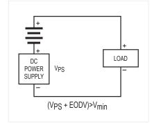
Figure 7. Using an Offset dc Power Supply
