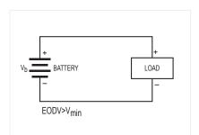
Figure 5. Single Battery Test Configuration
