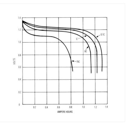
Figure 3. Effect of Discharge Rate on Capacity
