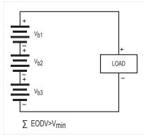
Figure 6. Batteries in Series
