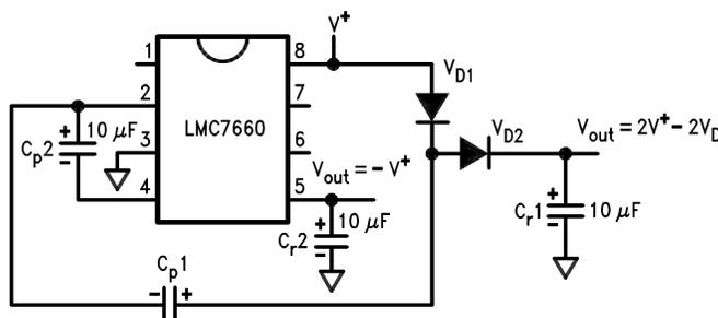
Figure 19. Combined Negative Converter and Positive Multiplier
