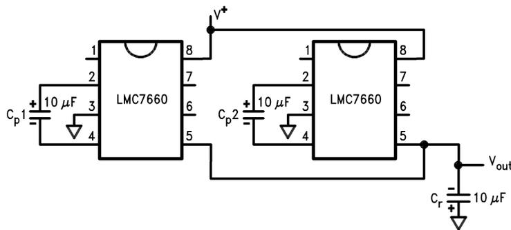
**Figure 14. Lowering Output Resistance by Paralleling Devices**
