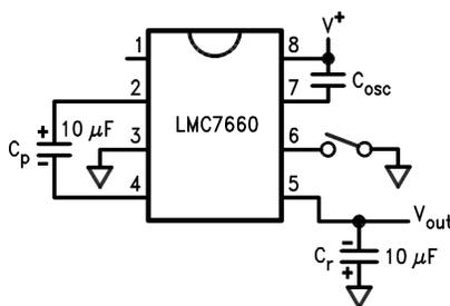
Figure 12. Reduce Supply Current by Lowering Oscillator Frequency
