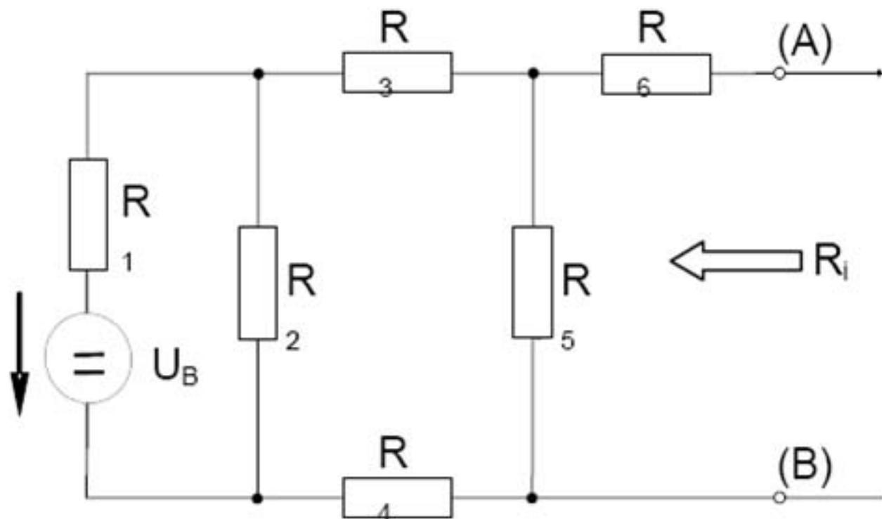
$$R_i = R_6 + [R_3 + R_1 \parallel R_2 + R_4] \parallel R_5$$
