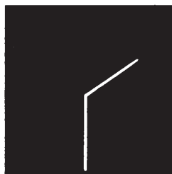
Diode paralleled by 680 \Omega
