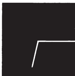
Diode in series with 51 \Omega
