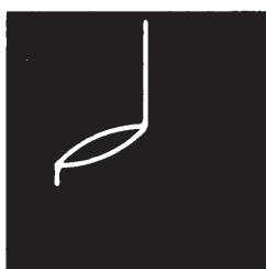
B-E with 1 \mu\text{F} + 680 \Omega
