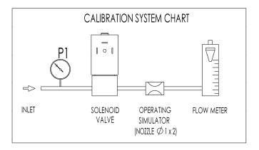
V164B02 – ZE30A (orifice size=1.6mm)
