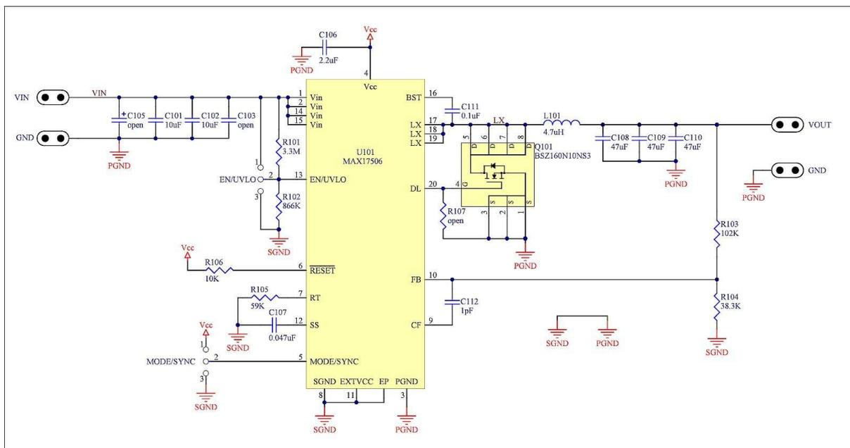
**Figure 1** Final design for +3.3V, 16.5W step-down converter
