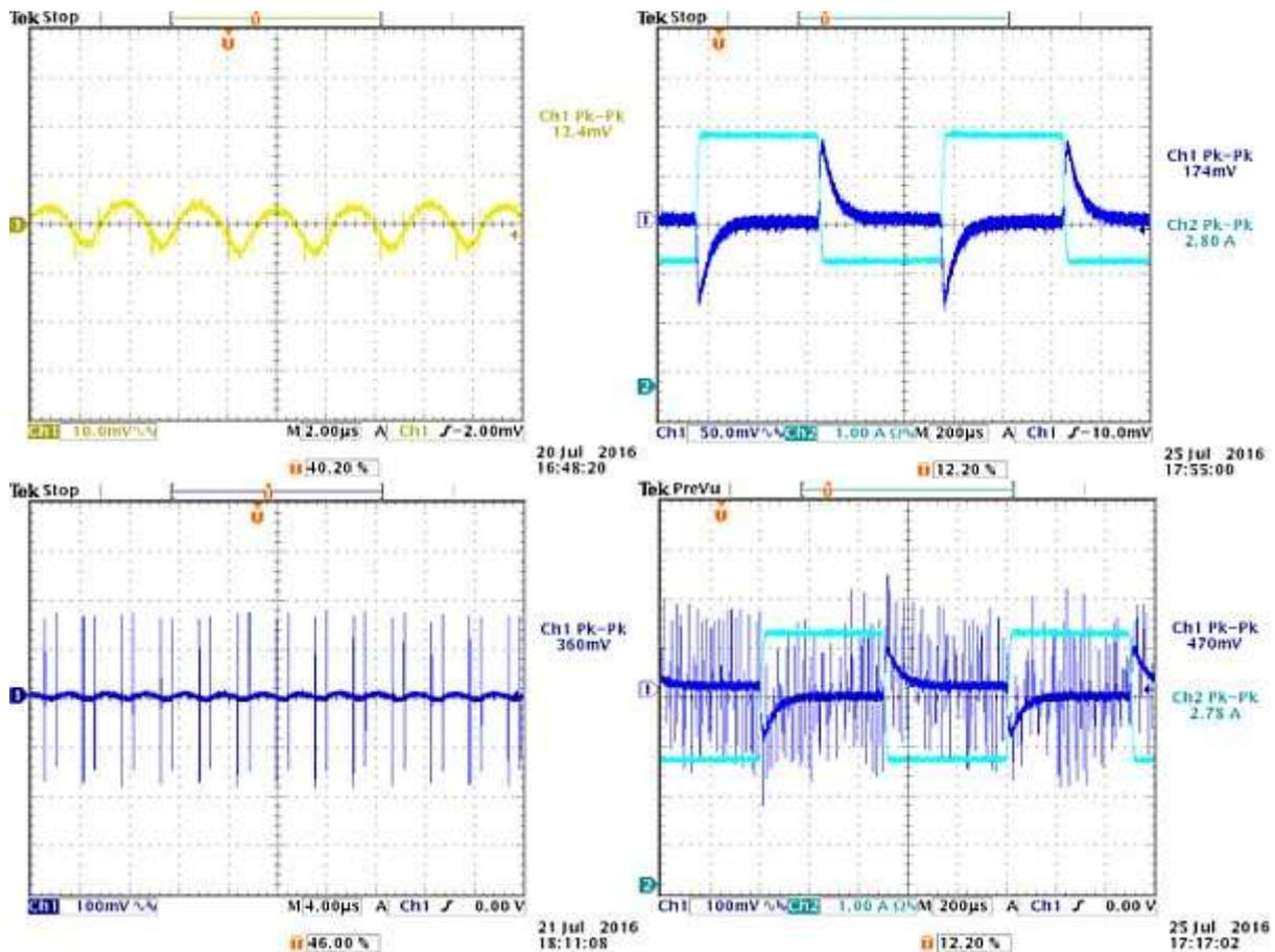
**Figure 12** Differences in measured waveforms between optimal layout (top) and narrow-trace layout (below)
