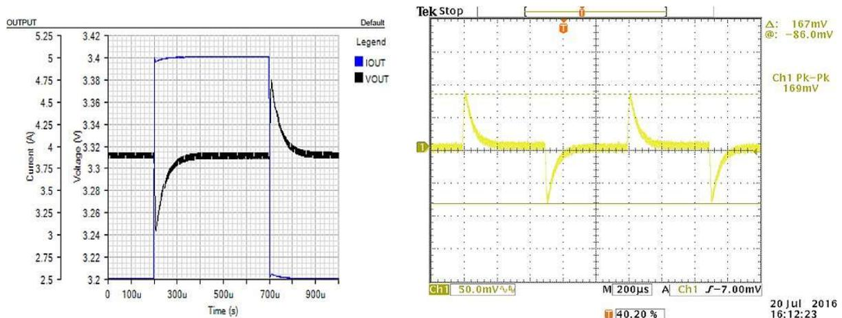
**Figure 4** Simulated load transient response (left) versus achieved response (right).
