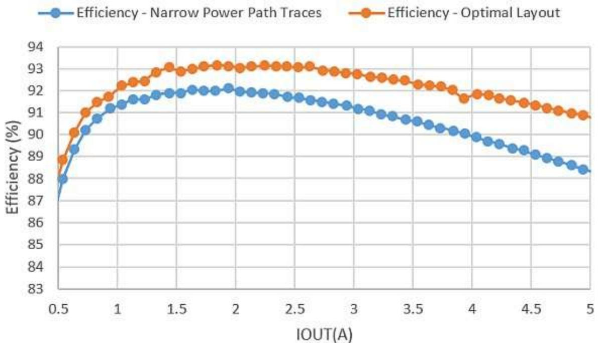
**Figure 11** Efficiency drop in narrow-traces layout versus optimal layout board
