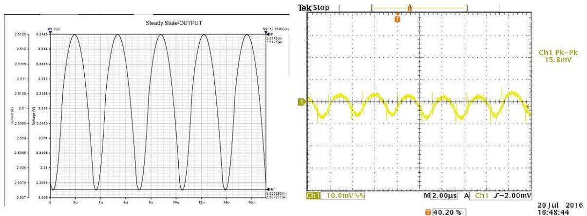
**Figure 5** Simulated (left) versus measured (right) output ripple with 2.5A load
