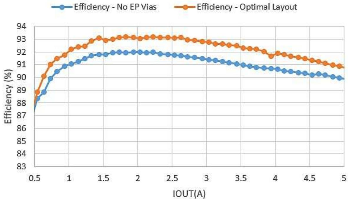
**Figure 8** Decreased efficiency in layout without exposed paddle vias
