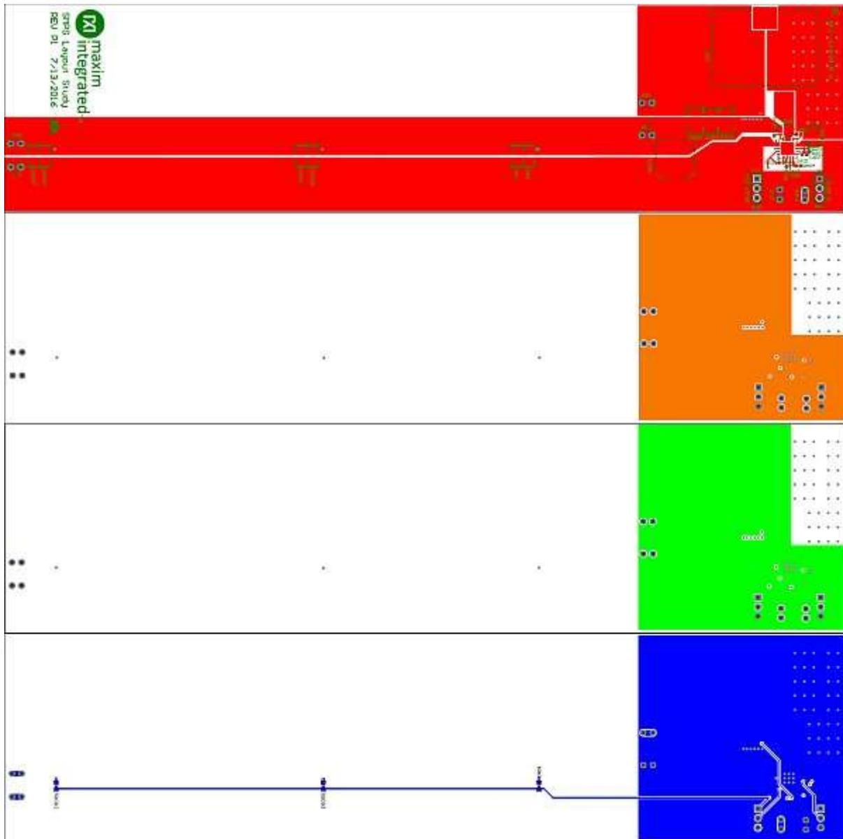
**Figure 18** Layout modified to show remote input capacitor placement
