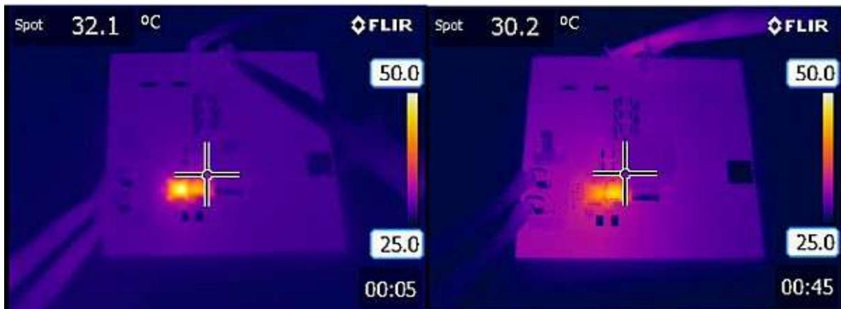
**Figure 9** IC temperature on no-EP-vias board (left) versus IC temperature on optimal layout board (right)
