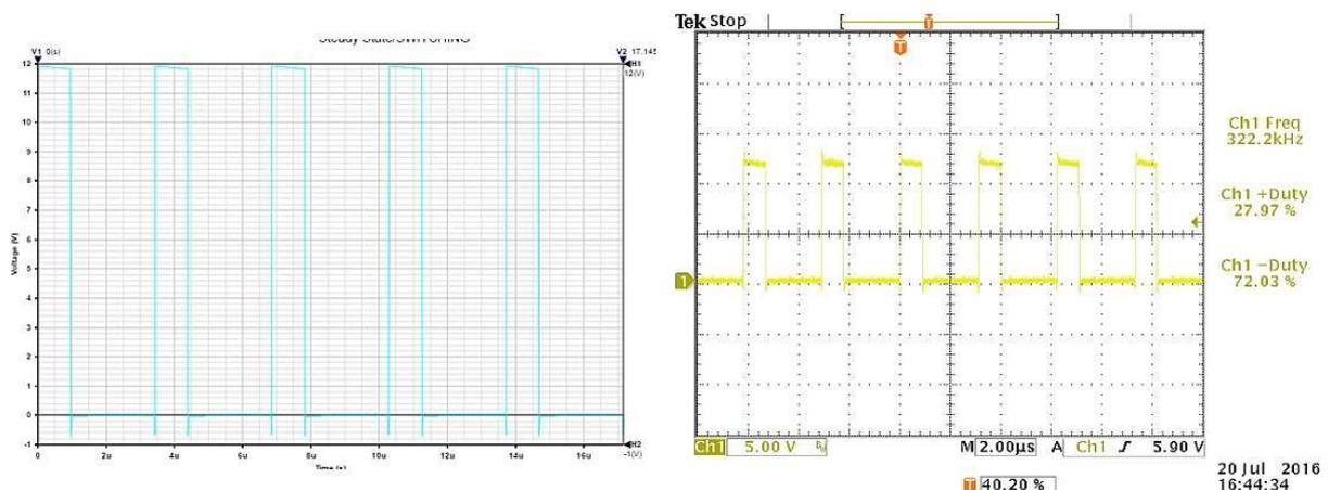
**Figure 6** Simulated (left) versus measured (right) switching-node waveforms
