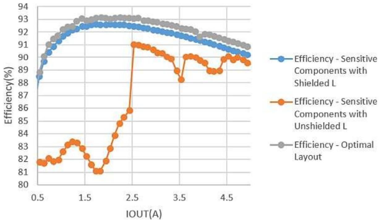
**Figure 14** Efficiency impact from moving sensitive analog components
