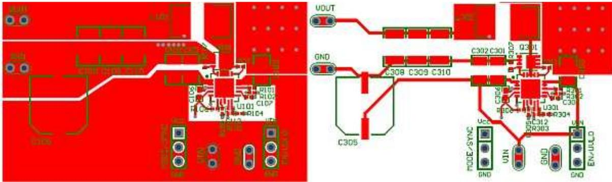
**Figure 10** Optimal top-layer layout (left) versus modified top-layer layout (right)
