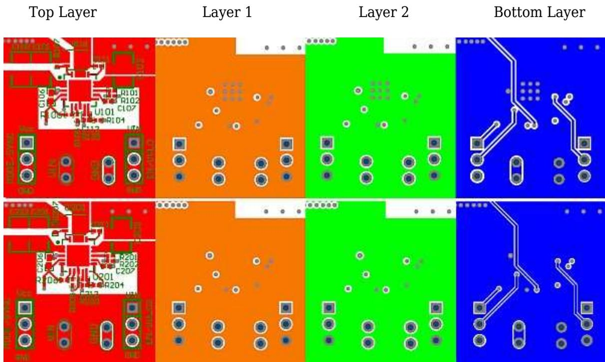
**Figure 7** Close-up of layout modification on MAX17506. Optimal layout (top layer) versus no EP pad layout (bottom layer).
