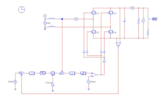
The simulation circuit shows the principle of the bidirectional VSI. The input stage consist of two half bridge IGBT with internal fast freewheeling diodes. On the input side are the two boost inductions (each 2mH). The value of the DC-BUS capacitor is 5000uF. The controller consist of a voltage controller (PI) and a current controller (PI).
