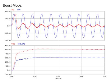
At the beginning (VDC<VAC<sub>peak</sub>) the input bridge is working as a normal passive rectifier. The inrush current is limited to 300A only by the boost induction. After aprox. 20ms the boost controller starts to boost the bus voltage to 500V, the input current is purely sinusoidal. With the VSI a high power factor with very low THD is achieved.
