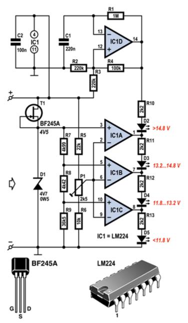
We'll use a simple quadruple <u>opamp</u> chip for the four comparators (IC1A..IC1C). The output turns high (i.e. equal to the supply voltage) as soon as the voltage on the plus input is even slightly higher than the voltage on the minus input, and low if the minus input is higher than the plus input, due to the extremely high amplification factor of a non-inverting opamp. This property lets an opamp mimic a comparator.
