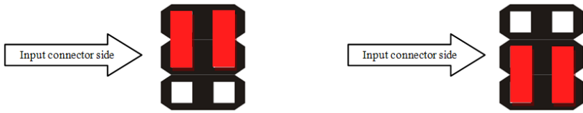
Figure 2: Jumpers' position. Left ( \pm 1 V full scale), right ( \pm 20 V full scale)
