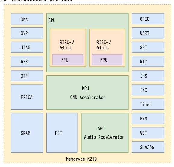
The K210 includes two 64-bit RISC-V CPU cores, each with a built-in independent FPU. The primary functions of the K210 are machine vision and hearing, which includes the KPU for computing convolutional neural networks and an APU for processing microphone array inputs. The K210 features a Fast Fourier Transform (FFT) Accelerator for high performance complex FFT calculations. As a result, for most machine learning algorithms, the K210 has high-performance processing power.
