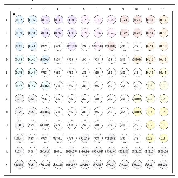
The pin definition of the chip is as shown above (top view, solder balls facing downwards). The chip is packaged in a BGA144, square, with 12 pins on each side. The chip has a width of 8mm, a length of 8mm and a height of 0.953mm.
