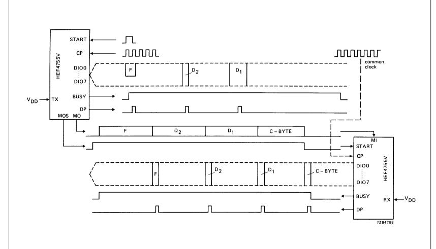
Function/timing diagram when using the HEF4755V in the asynchronous mode where the byte number per message is variable and the hamming distance is 4.
