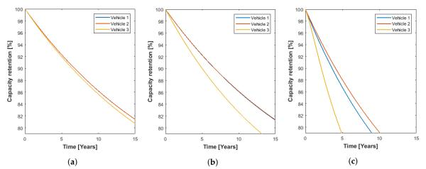
**Figure 9.** Ageing for the three vehicles while assuming driving according to, (a) WLTC medium; (b) WLTC; and (c) WLTC Extra High for five full charge/discharges per week all year around with a battery temperate of 30 °C.
