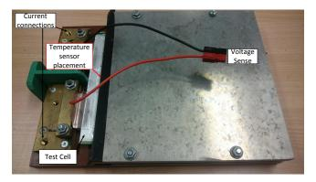
Figure 1. Test cell with holder.
