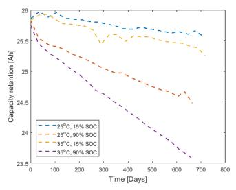
Figure 3. Calendar ageing in 25 °C and 35 °C at 15% and 90% State of Charge (SOC).
