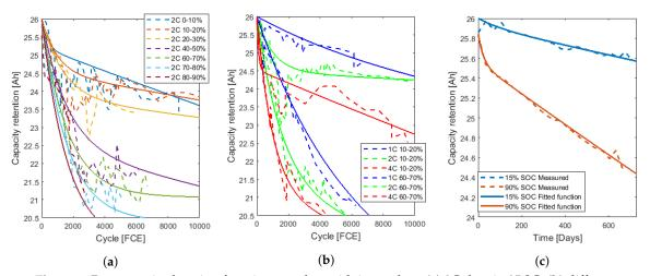
**Figure 5.** Parameterised ageing function together with input data, (a) 2C data in 25  $^{\circ}$ C; (b) different C-rates in 35  $^{\circ}$ C; and (c) calendar ageing in 25  $^{\circ}$ C at 15% and 90% SOC and the corresponding degradation equations.
