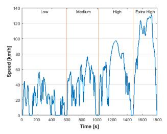
**Figure 7.** The Worldwide Harmonized Light Vehicles Test Cycle (WLTC) drive cycle for Class 3b vehicles used to estimate the energy consumption [13].
