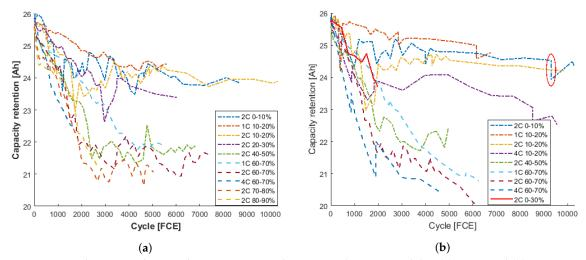
**Figure 2.** The ageing data used to parameterise the empirical ageing model in (a) 25 °C and (b) 35 °C. In (b), the data is also used to verify the model included. The vertical changes in capacity indicates stops in the testing due to maintenance, i.e., a rest period.
