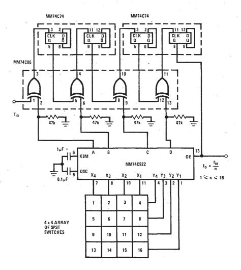
Simply press the key and the input frequency is divided by that number. The output frequency is symmetrical for odd and even divisors. Use it for simple frequency synthesis or as a keyboard controlled oscilloscope triggering unit.
