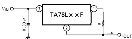
$$I_{OUT} = \frac{V_{OUT}}{R} + I_B$$
