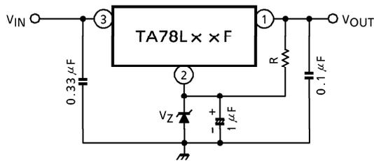
$V_{OUT} = V_Z + V_{OUT}(\text{of IC})$
