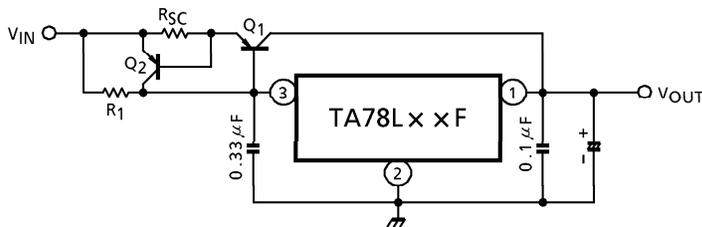
$$R_{SC} = \frac{V_{BE2}}{I_{SC}}$$
