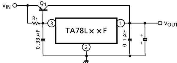
Use a required radiation plate for Q<sub>1</sub>.
