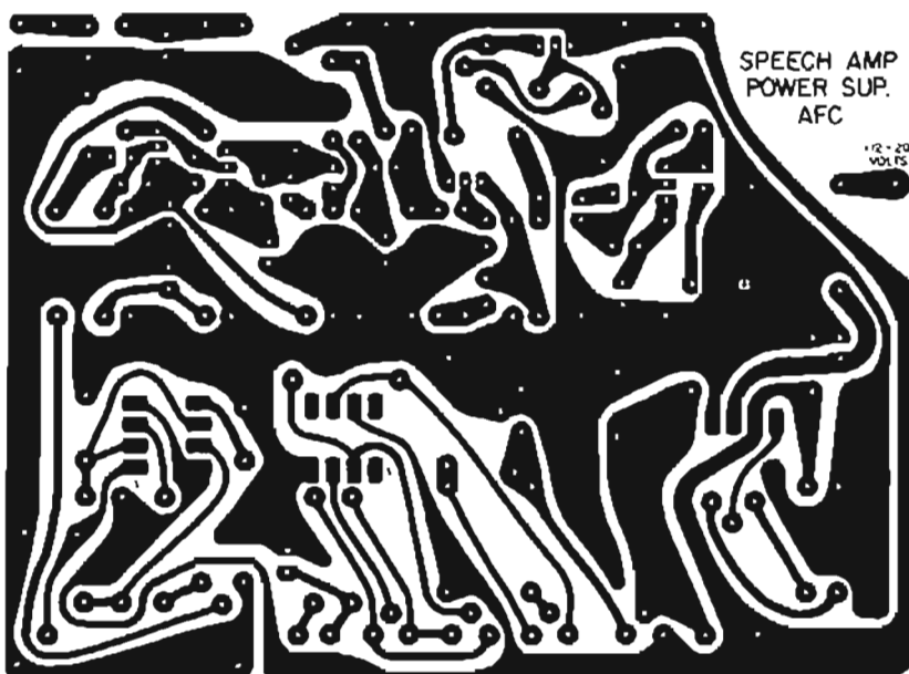
fig. 23. Full-size printed-circuit layout for the Gunnplexer speech amplifier, tone oscillator, AFC amplifier, and voltage regulator. Component layout is shown in fig. 22.
