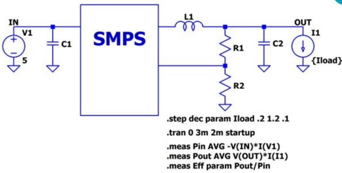
The `.step` command is useful for sweeping a variable across a range of values in a single simulation run. The variable can be temperature, a model parameter, a global parameter or in our case an independent source. These steps can be defined as linear, logarithmic or as a list of specific values.
