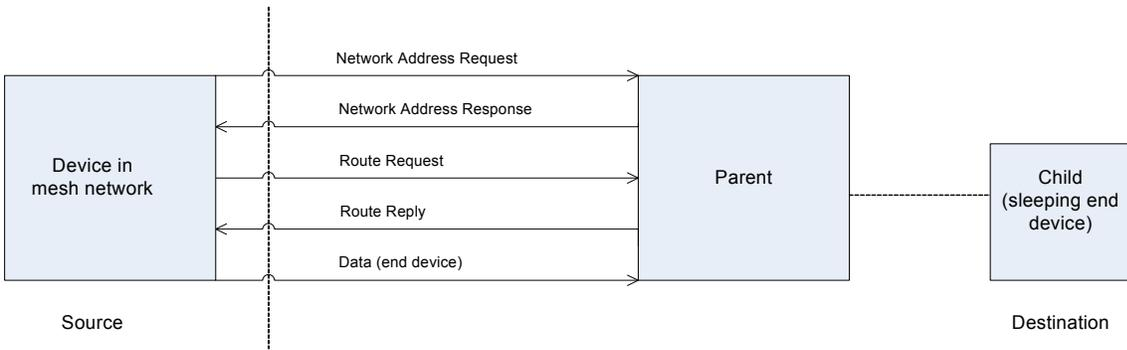
**To talk to an end device, a source device in a mesh network must talk to the parent to determine the address and the route of the end device. The source device then sends data to the parent.**
