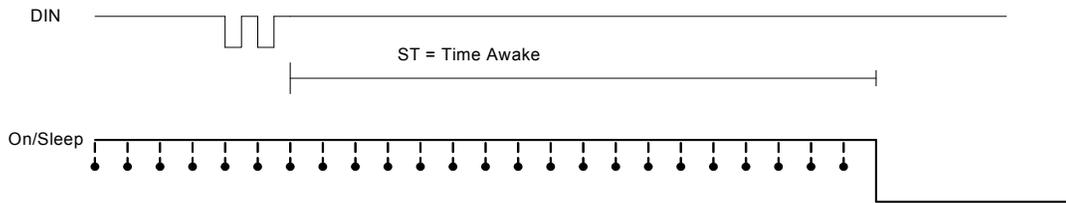
**A cyclic sleep end device enters sleep mode when no serial or RF data is received for ST time.**
