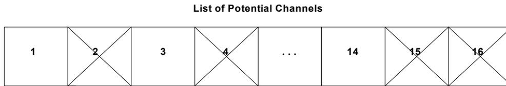
Performing an energy scan allows the coordinator to avoid starting on channels with high energy levels.
