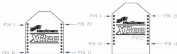
**Table 1-02. Pin Assignments for the XBee PRO ZNet 2.5 Modules**
