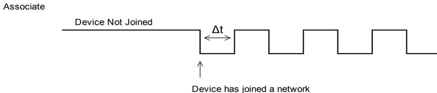
**The associate pin can indicate the joined status of a device . Once the device has joined a network, the associate pin toggles state at a regular interval ( $\Delta t$ ). The time can be set by using the LT command.**
