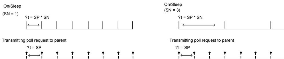
Setting SN > 1 allows the XBee to silently poll for data without asserting On/Sleep. If RF data is received when polling, On/Sleep will immediately assert.
