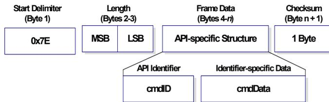
The cmdID frame (API-identifier) indicates which API messages will be contained in the cmdData frame (Identifier-specific data). Note that multi-byte values are sent big endian. The XBee ZNet 2.5 modules support the following API frames:
