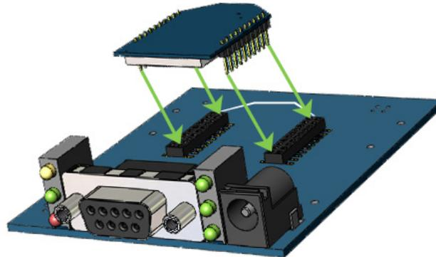
The receptacles used on Digi development boards are manufactured by Century Interconnect. Several other manufacturers provide comparable mounting solutions; however, Digi currently uses the following receptacles:
