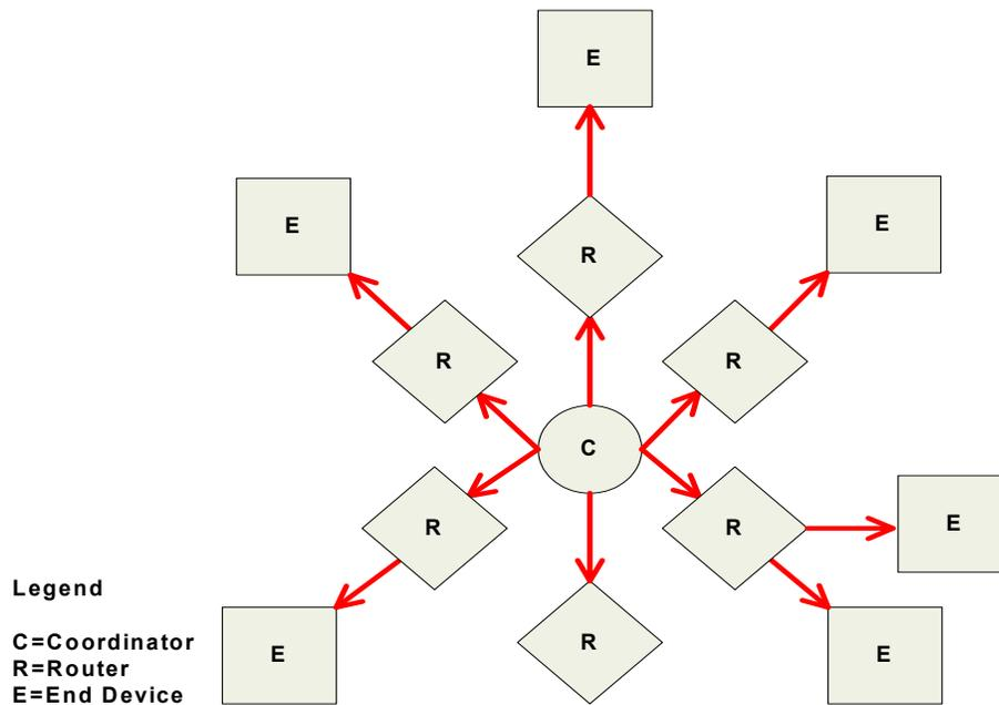
Each node that transmits the broadcast will also create an entry in a local broadcast transmission table. This entry is used to keep track of each received Zig broadcast packet to ensure the packets are
