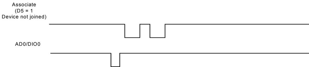
**A single commissioning button press when the device has not joined a network that causes the associate pin to blink to indicate the AI Code where: AI = # blinks + 0x20. In this example, AI = 0x22.**
