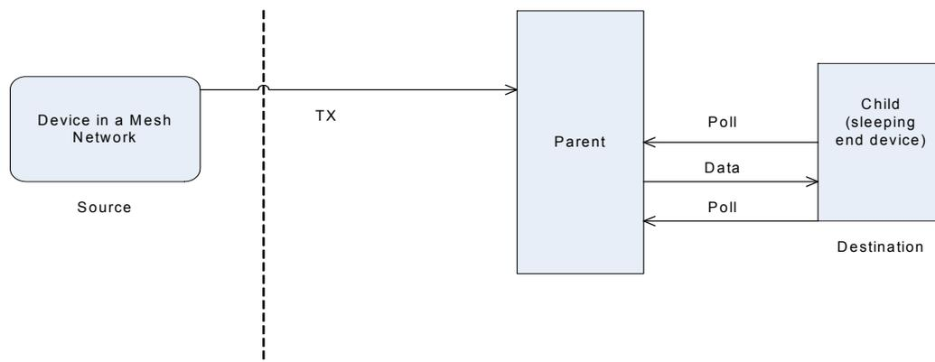
**When RF data is sent to a sleeping end device, the end device's parents buffers the data until the end device polls for the data, or a timeout occurs**
