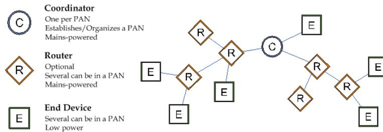
**Coordinator** – Responsible for selecting the channel and PAN ID. The coordinator starts a new PAN. Once it has started a PAN, the coordinator can allow routers and end devices to join the PAN. The coordinator can transmit and receive RF data transmissions, and it can assist in routing data through the mesh network. Coordinators are not intended to be battery-powered devices. Since the coordinator must be able to allow joins and/or route data, it should be mains powered.
