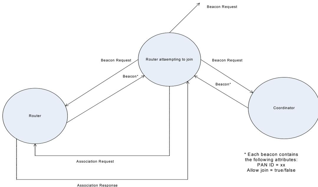
A router or end device sends a beacon request to discover nearby Zigbee networks. If a device is found that is operating on a valid Zigbee network, that is allowing joins, the router or end device sends an association request to that device to attempt to join the network
