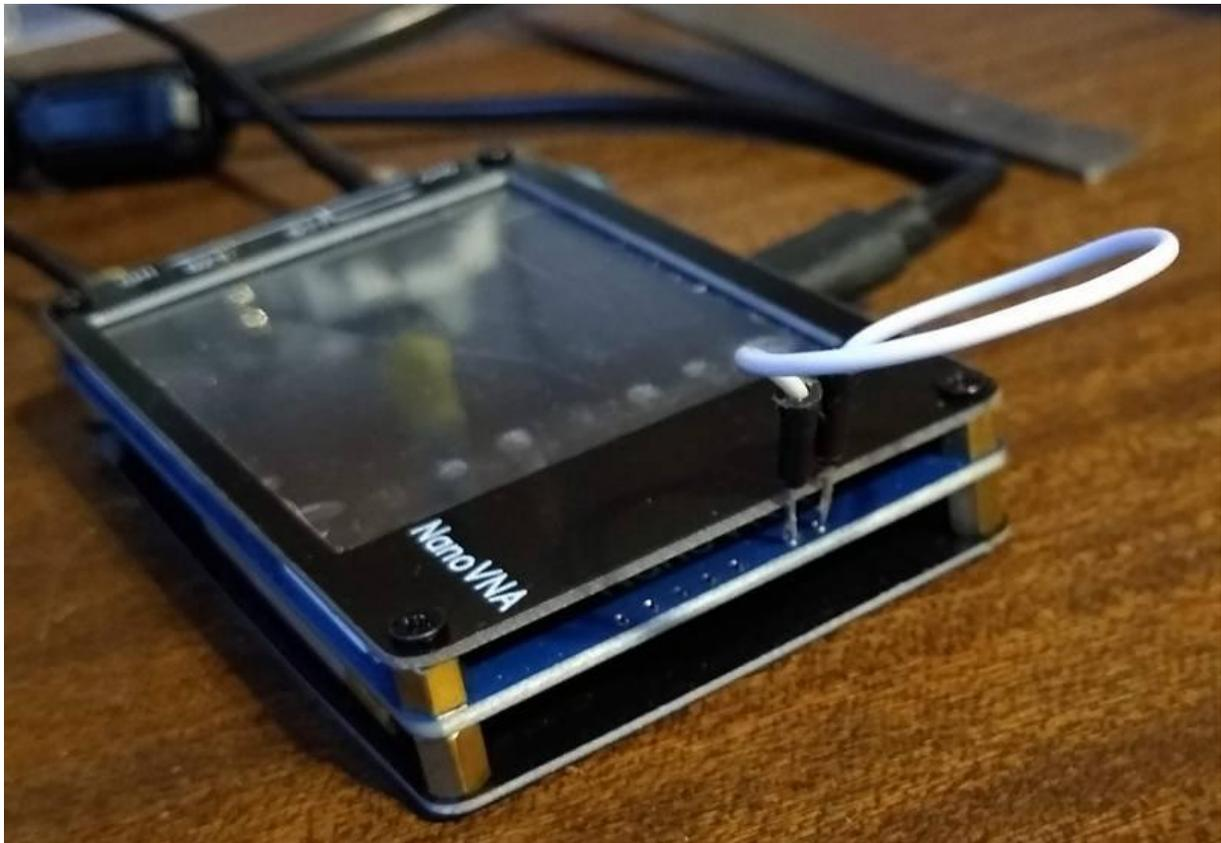
Connect the two rightmost holes, NOT any holes to the left, with a standard Dupont cable or any cable that has small pins that will fit into the holes in the board. Do NOT use force. You may have to bend the pins a little to be able to insert them
