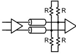
Although the single resistor termination to  $V_{TT}$  conserves power, it requires an additional supply voltage. An alternate approach to using a  $V_{TT}$  power supply is to use a resistor divider network as shown in Figure 12 to develop a Thevenin voltage,  $V_{TT}$ , and provide a parallel impedance matching AC termination, the Thevenin parallel termination.
