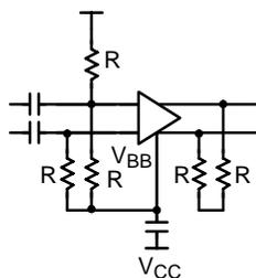
Although not strictly a termination, AC or capacitive coupling is often used to provide features in conjunction with proper termination. Such capabilities as hot swapping capability, DC isolation to a receiver, and level shifting are possible with capacitive coupling.
