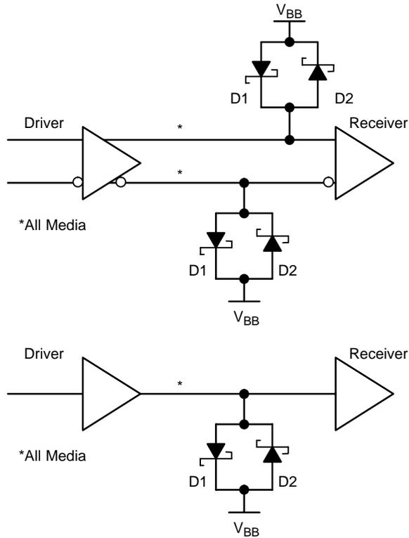
Figure 19. Diode Termination
