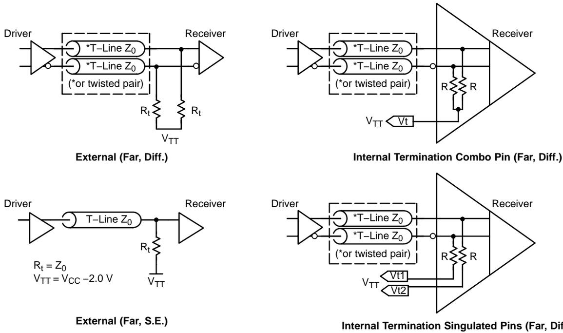
**Figure 4. Parallel Termination to  $V_{TT}$  – Differential and Single-Ended with Combo or Singulated  $V_t$  Pins (Far Return) Internal Termination Resistors**
