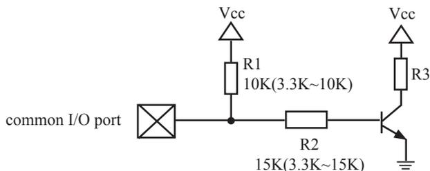
If I/O is configed as “weak” pull-up, you should add a external pull-up resistor R1(3.3K~10K ohm). If no pull-up resistor R1, proposal to add a 15K ohm series resistor R2 at least or config I/O as “push-pull” mode.
