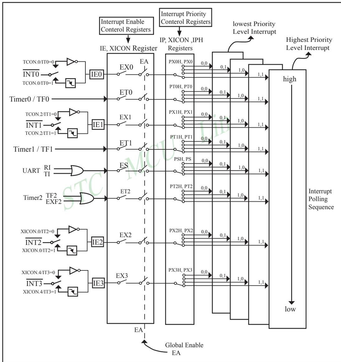
Figure STC89C51RC/RD+ series Interrupt Structure diagram
