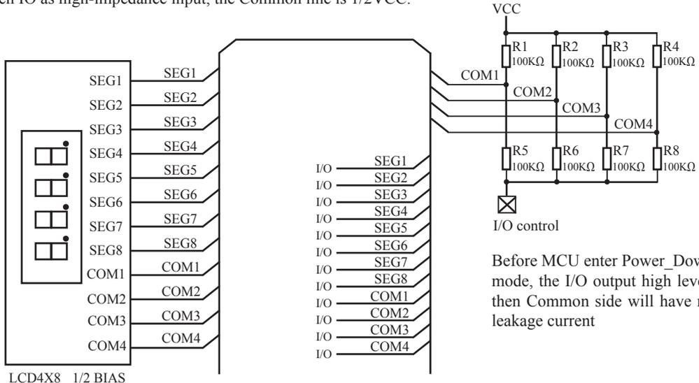
Before MCU enter Power\_Down mode, the I/O output high level, then Common side will have no leakage current
