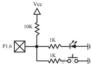
It can save a lot of I/O ports that STC89C51RC/RD+ MCU I/O ports can be used as the LED drivers and key detection concurrently because of their feature which they can be set to the weak pull, the strong pull (push-pull) output, only input (high impedance), open drain four modes.
