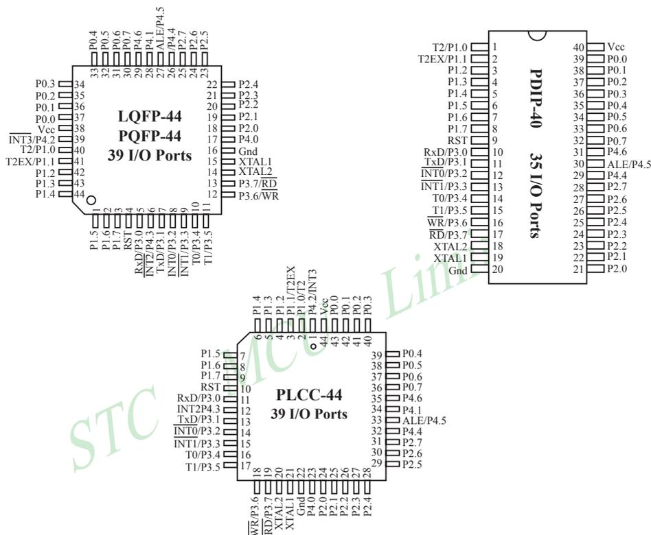
About operation voltage/clock frequency: RC/RD+ series MCU are real 6T MCU, which are full compatible with traditional 12 clocks per machine cycle
