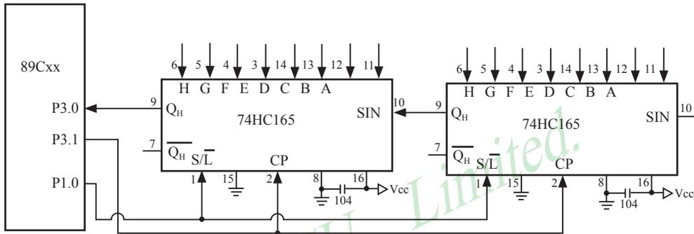
74HC165 is a 8-bit parallel input shift register, when S/L (Shift/Load) pin is falling to low level, the parallel port data is read into internal register, and now, if S/L is raising to high and ClockDisable pin (15 pin) is low level, then clock signal from CP pin is enable. At this time register data will be output from the Dh pin (9 pin) with the clock input.
