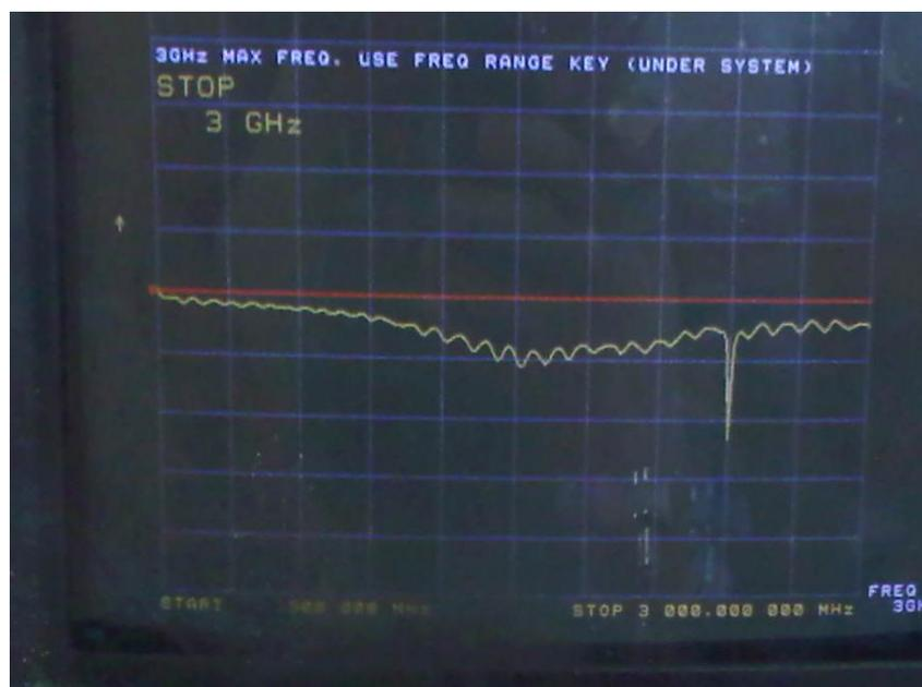
3. Connect screw  $S_2$  next to  $S_1$  (arbitrary distance) and tune until two peaks are visible on the screen.
