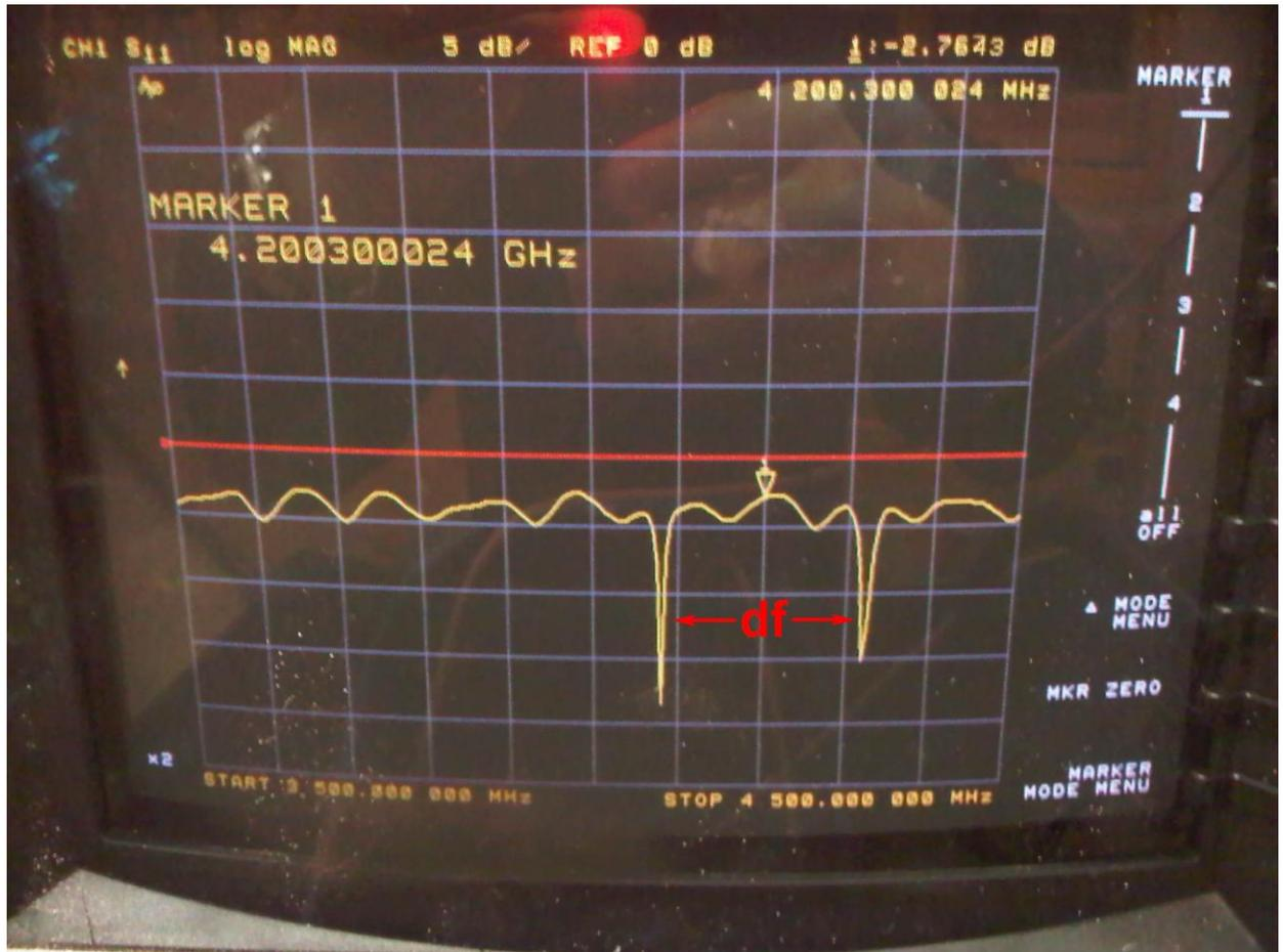
4. Move  $S_2$  and repeat measurement, until enough data is obtained in order to plot coupling curve. The farther  $S_2$  is from  $S_1$ , the smaller the peaks (dibs) will be, since the signal is being attenuated fast.
