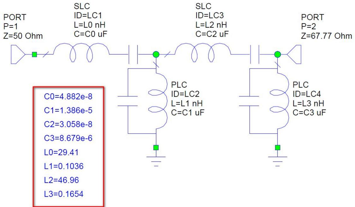
The L and C values in the circuit were calculated using the filter transformation equations mentioned earlier, with the published g-values for a 4-pole, 0.1 dB Chebyshev ripple [5].
