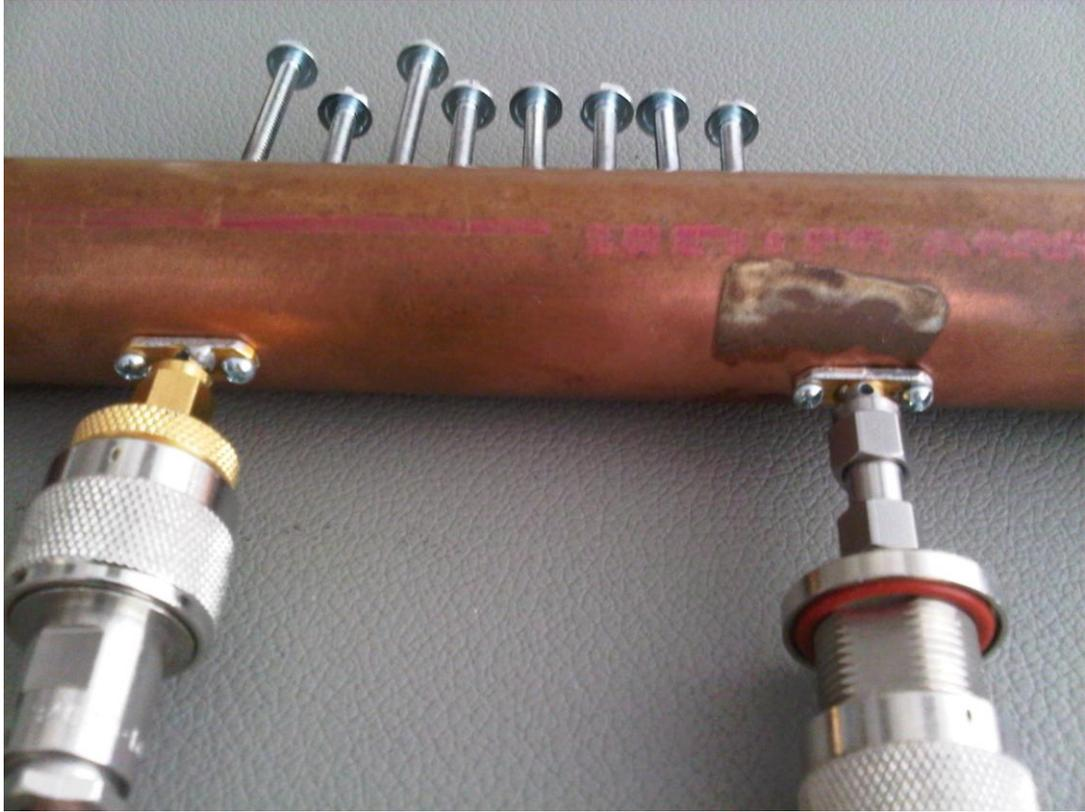
5. Tuning the filter – for 0.1 dB ripple, need to achieve  $\approx 16$ dB Return Loss
