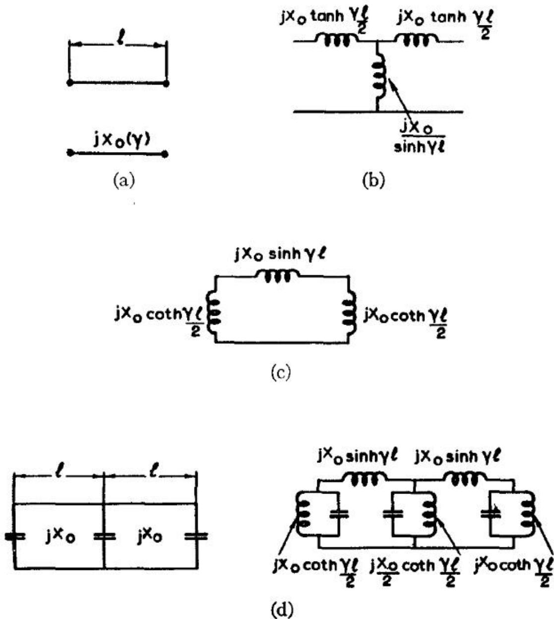
Fig. 1. (a), (b), and (c) Equivalent circuits of evanescent mode waveguide. (d) Lumped equivalent circuit of evanescent mode waveguide filter.
