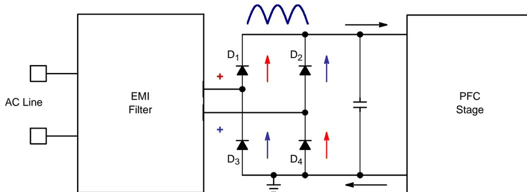
Figure 1. The Input Current Flows Through Two Diodes
