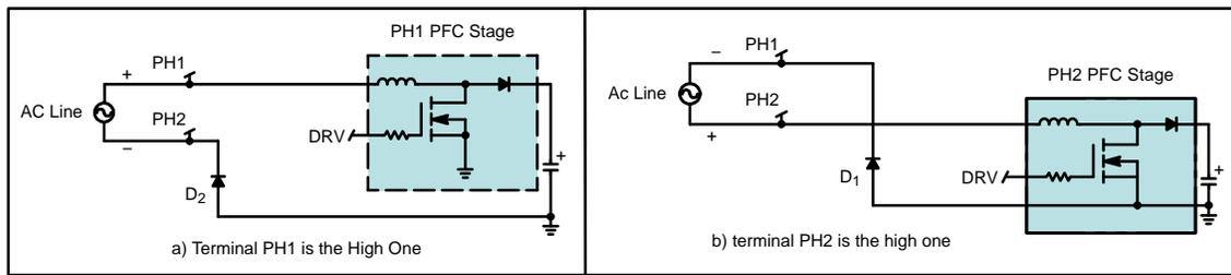
Figure 7. Equivalent Schematic for the Two Half-Waves
