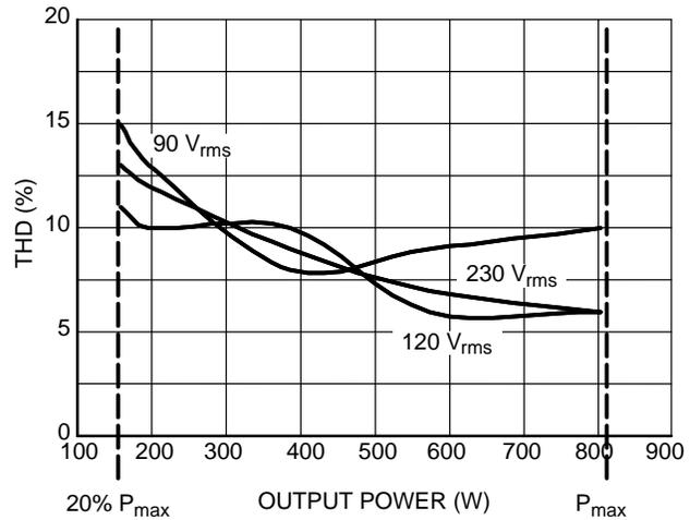
**Figure 16. Total Harmonic Distortion Over the Load Range**
