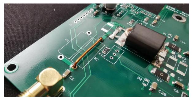
R1 and R2 can fit 3W resistors (2 or 3 can be stacked in each position for more power handling) and R3 is a 2512 SMD resistor typically rated at 1W, so keep that in mind when you design your attenuator. If you have less than 5W drive or you plan to use an off-board attentuator, just install the straight wire in place of R2. No need to worry about its inductance as the capacitor at T1's input cancels it.
