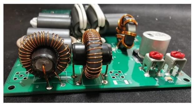
L1 - 8 turns bifilar on toroid. Cut the supplied wire in two equal lengths and wind the two wires together on the toroid; it should be enough for 8 turns, with a bit to spare. With the utility knife scrape the insulation from the wire ends.
