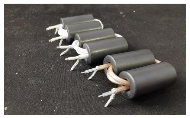
Quicky coat in solder the exposed shielding and the central wire and then solder in place. Do not heat more than necessary as it may damage the coaxial cable.
