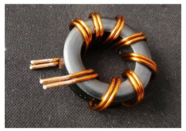
Make sure you apply a clean layer of solder coating, install L1 as in the picture and solder in place.
