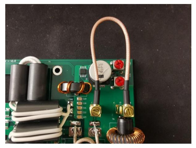
Slowly turn RV1 so the Gate voltage increases until the total board current has increased by 200mA (for example to 240mA if the initial drain was 40mA). Do the same for RV2 until the current has increase by another 200mA.
