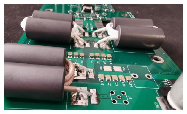
T6 & T7 - 33 turns on toroid with one central wire. Pay extra attention to symmetry with these two transformers, as it may affect forward & reflected power measurement in the higher frequencies. First, wind 33 turns of the thin wire on the toroid, as equally spaced as possible and making sure they cover about 90% of the toroid. Carefully scrape the insulation off the wire ends with the utility knife and coat in solder.
