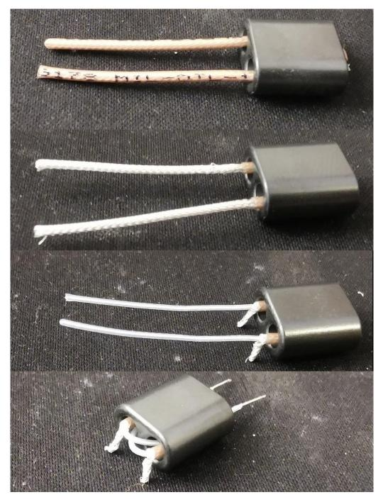
T3, T4 & T5 - 3 turns coaxial on two large ferrite cores. T3/T4 coax and ferrite cores have different specs than T5 so make sure you don't mix them. Wind the supplied coaxial cable so it passes 3 times through each of the two cores. With the utility knife remove the outer jacket over the last 1cm (1/2 inch) at each end, remove the shielding over the last 5mm (1/4 inch) and carefully cut the insulation to expose the tip of the central wire.
