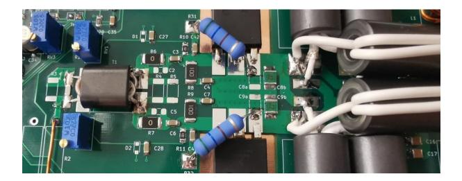
Now you can apply +48V again to the board and monitor current, which should still be around 40mA. Slowly turn RV1 so the Gate voltage increases until the total board current has increased by 200mA (for example to 240mA if the initial drain was 40mA). Do the same for RV2 until the current has increased by another 200mA.
