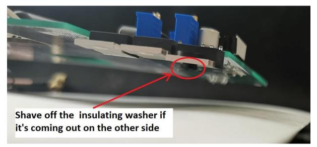
Place the heat spreader on the heatsink and the PCB on top of the heat spreader and screw down the four M4 bolts and then the three M3 bolts for U2, U3 and U4.
