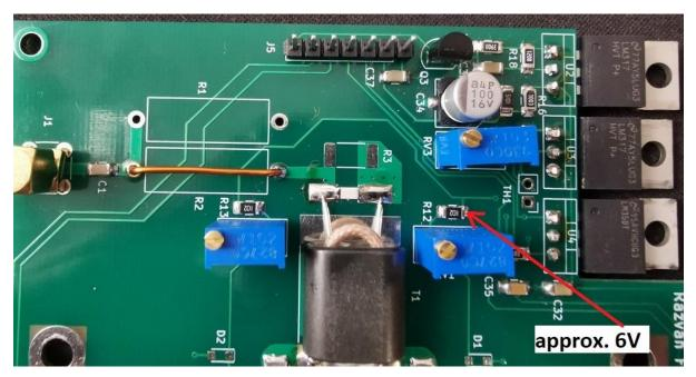
Measuring the voltage at the Gate pad for Q1, adjust RV1 until the voltage is around 2.2V and do the same for RV2 while measuring the Gate tab of Q2.
