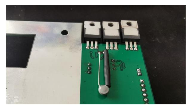
At this stage, place the PCB on the heatsink and check there is no protrusion on the back that could touch the heatsink, except TH1. Pay close attention to where L1, T6, T7 come through the board on the back as their traces carry a lot of energy. Remember there is only 3mm of spacing, provided by the copper heat spreader.
