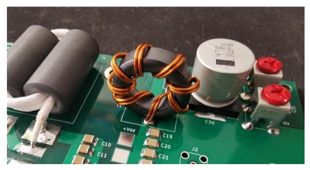
L2 & L3 - 3 turns on large ferrite bead. Wind the supplied wire so it passes 3 times through the ferrite core. Use the utility knife to remove about 5mm (1/4 inch) of wire jacket, coat with solder.
