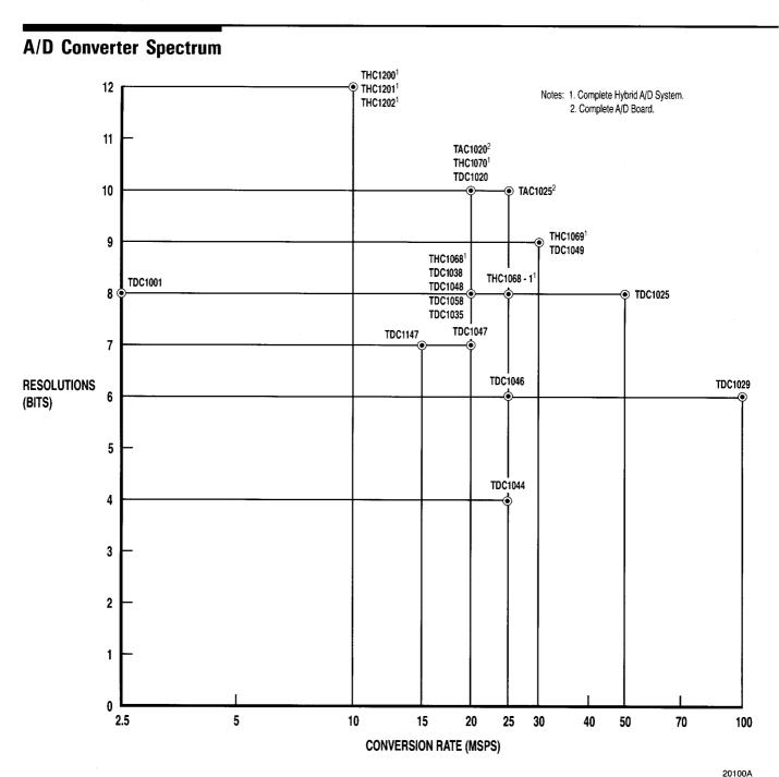
**A/D Converters** — TRW LSI's high-speed analog-to-digital converters utilize flash, two-pass and successive approximation architectures encompassing resolution from 4 to 12 bits and conversion rates from 2.5 to 100MSPS. All monolithic A/D converters are built using TRW's proven 3D (Triple Diffused) bipolar technology while hybrids combine various technologies to provide complete analog-to-digital conversion systems.
