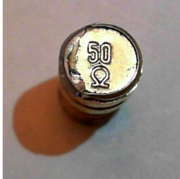
Step 6: Place to top lid and solder the milled away part
