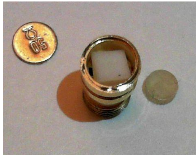
Step 6: Place to top lid and solder the milled away part
