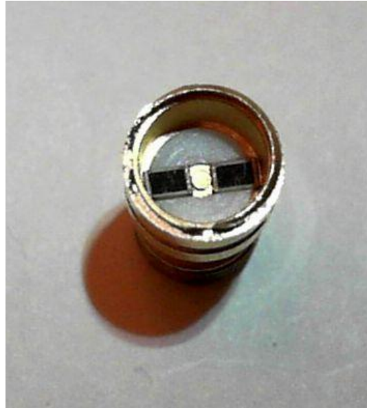
Step4: Place the third PAD without hole
