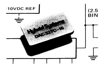
Analog outputs are short-circuit proof. Settling time for a full scale 10V step change to  $\pm 0.003\%$  F.S.R. is  $100\mu S$  and  $50\mu S$  for a 0.6mV change. Linearity is typically  $\pm 0.003\%$  F.S.R. for binary models and  $\pm 0.005\%$  F.S.R. for BCD models. Initially trimmed to  $\pm 10mV$ , offset may be externally adjusted if desired; models with built-in references can also be full scale adjusted by means of an external potentiometer.
