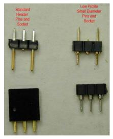
The standard header socket will work with HC-49 crystal leads, but the connection will not be nearly as solid as with the smaller socket. <sup>1</sup>/<sub>4</sub> watt resistor leads and many small capacitor leads will fit the standard socket, which extends the usefulness of the fixture.
