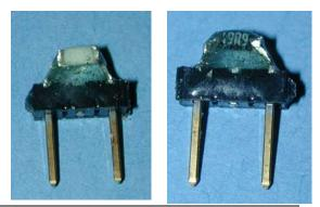
The result will be fragile; the resistor's ceramic substrate is easily broken. I use a small bit of 5-minute epoxy to encapsulate the resistor and mount to
