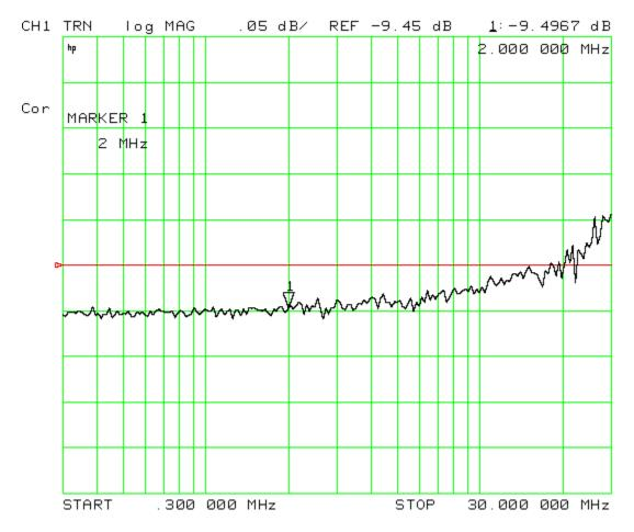
Using the same formula presented for the open socket case, using the measured attenuation of 9.4967 dB at 2 MHz, we calculate the resistance
