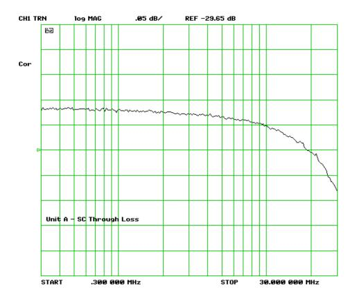
With the same test setup, remove the shorting bar. This measures the pad loss and the stray capacitance between the crystal socket pins.
