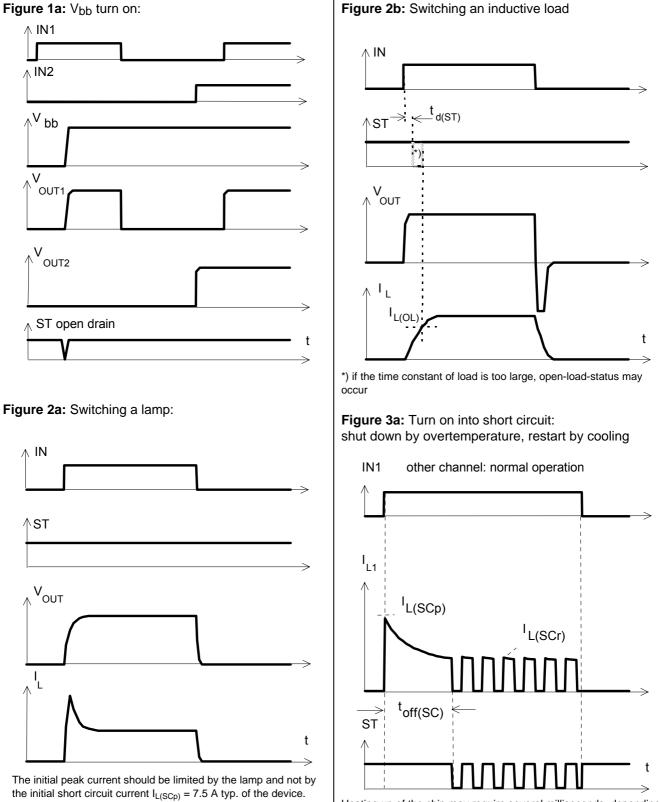
Heating up of the chip may require several milliseconds, depending on external conditions ( $t_{off(SC)}$  vs.  $T_{i,start}$  see page 11)
