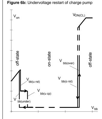
IN = high, normal load conditions. Charge pump starts at  $V_{bb(ucp)} = 5.6 V$  typ.
