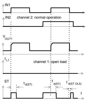
$t_{d(\text{ST OL5})}$  depends on external circuitry because of high impedance
