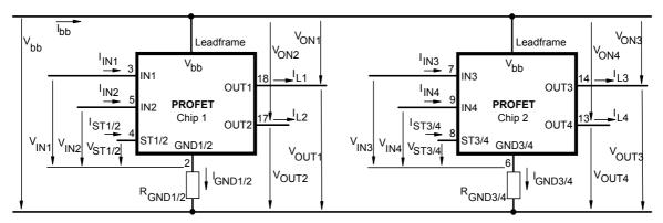
Leadframe (V<sub>bb</sub>) is connected to pin 1,10,11,12,15,16,19,20 External R<sub>GND</sub> optional; two resistors R<sub>GND1/2</sub>, R<sub>GND3/4</sub> = 150  $\Omega$  or a single resistor R<sub>GND</sub> =75  $\Omega$  for reverse battery protection up to the max. operating voltage.
