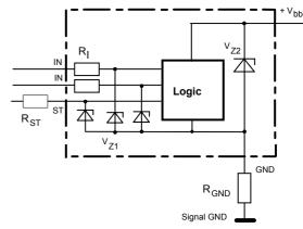
$V_{Z1}$  = 6.1 V typ.,  $V_{Z2}$  = 47 V typ.,  $R_I$  = 3.5 k $\Omega$  typ.,  $R_{GND}$  = 150  $\Omega$
