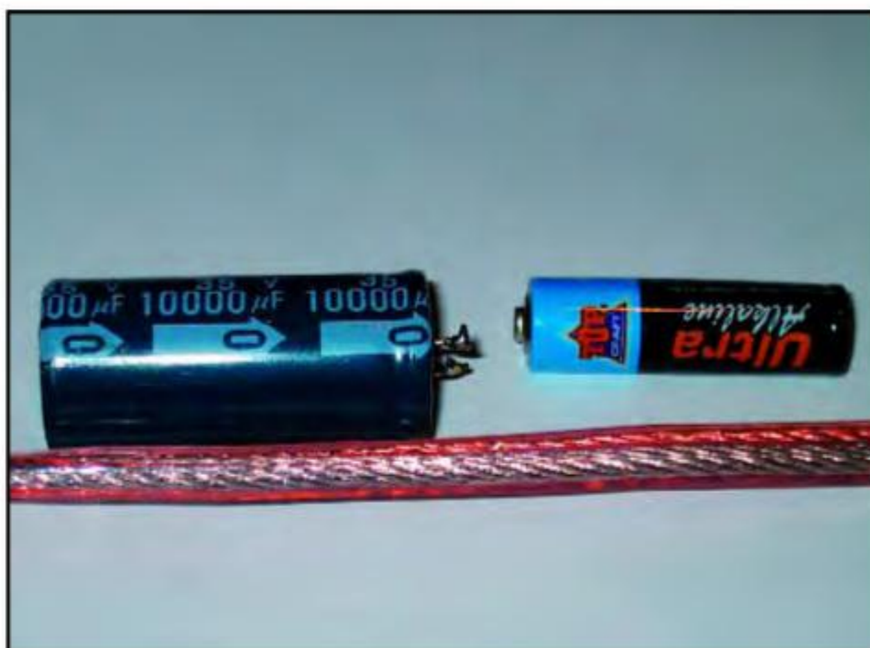
The main part: the capacitor. This is a 10,000 \mu\text{F} -version. Eight of these are tied together with thick loudspeaker cable (the battery is an AA penlite, for reference)
