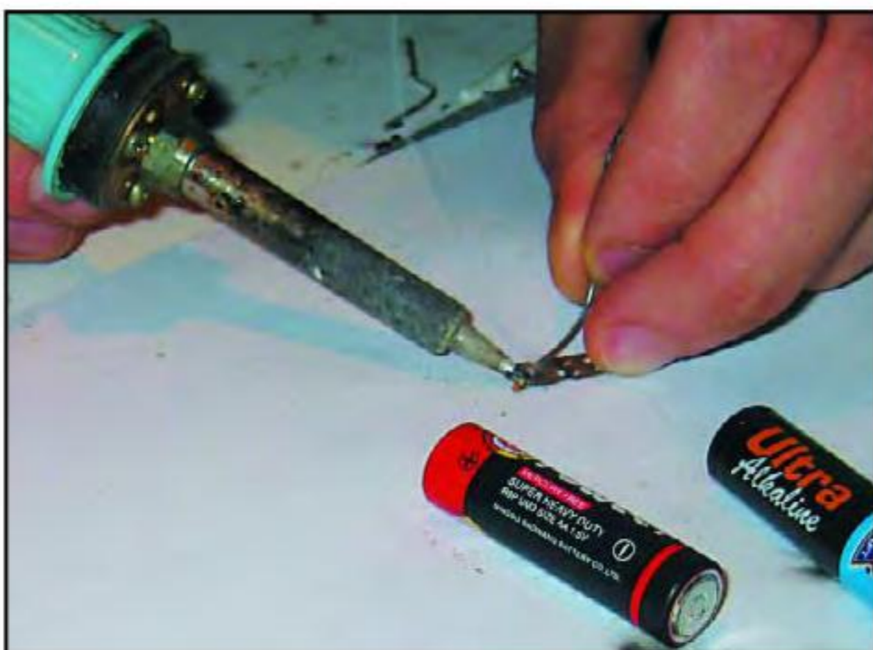
It helps to tin the metal well where it will be joined to the battery. Solder melts easier than the strip of metal or the metal end of the battery.
