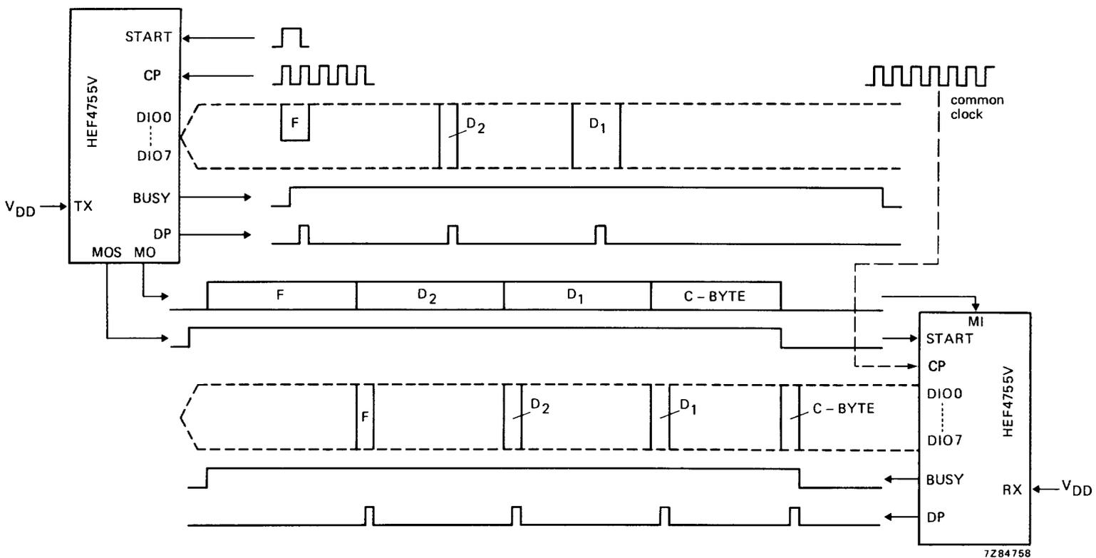
Fig.7 Function/timing diagram when using the HEF4755V in the asynchronous mode where the byte number per message is variable and the hamming distance is 4.
