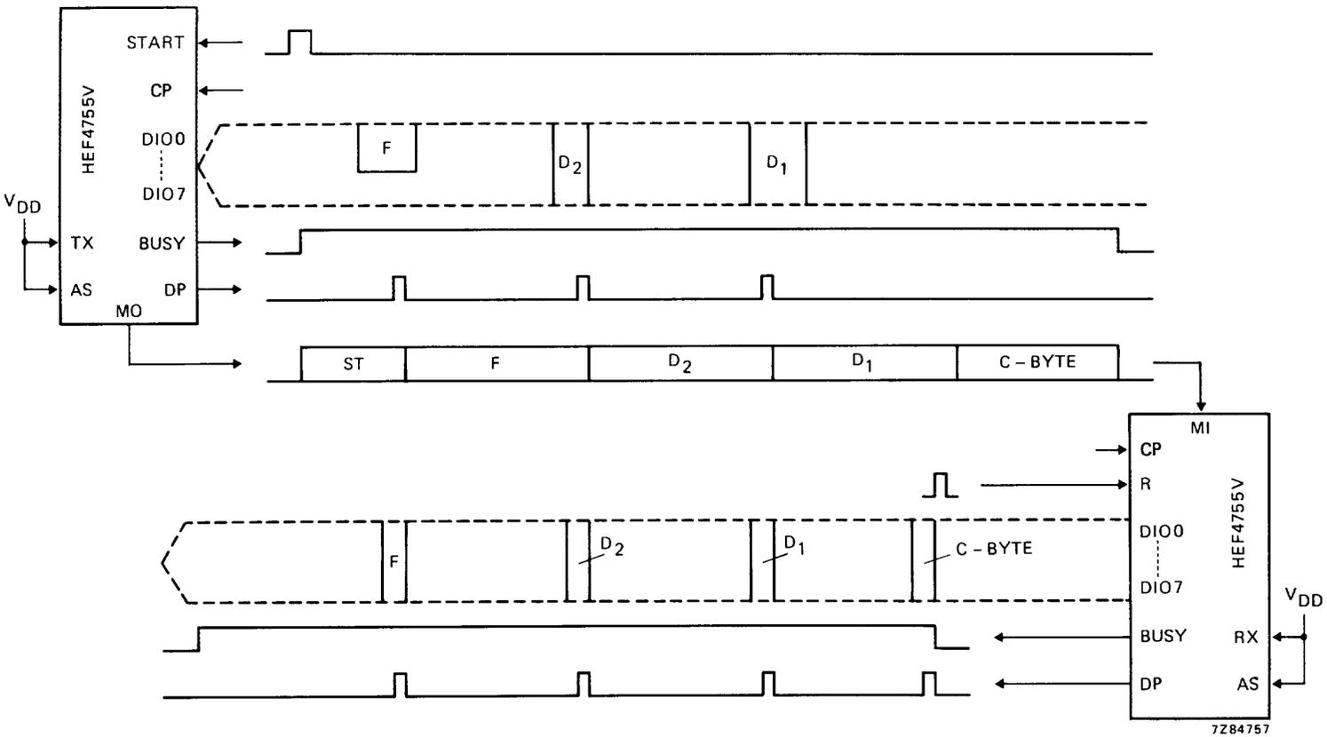
Fig.8 Function/timing diagram when using the HEF4755V in the asynchronous mode where the byte number per message is variable and the hamming distance is 4.
