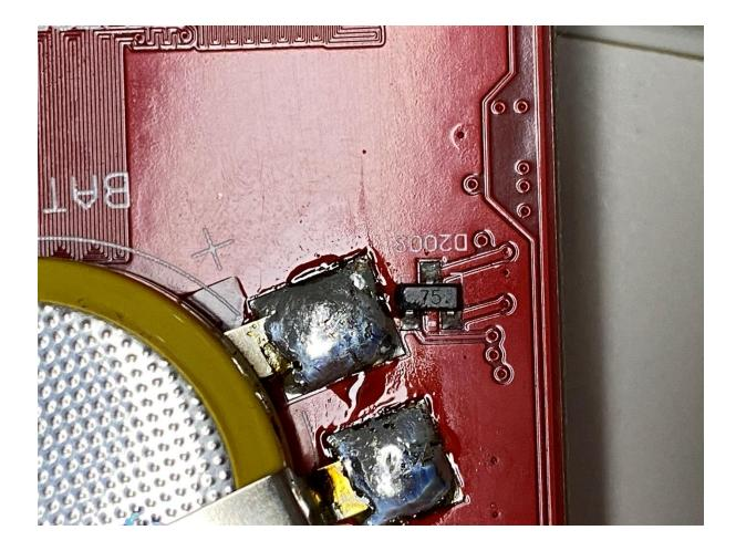
Metal stripes that are soldered onto the PCB making contact to Battery
