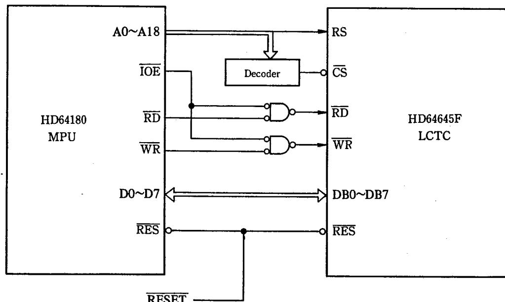
Note; Concerning 80 family MPU's, I/O space is separate from memory space in software. Thus the LCTC, a part of I/O, needs the ANDed signals of the interface signals and  $\overline{IOE}$ . So  $\overline{IOE}$  and  $\overline{RD}$ , and  $\overline{IOE}$  and  $\overline{WR}$  should be ORed to satisfy  $t_{AS}$ , the timing of  $\overline{CS}$ ,  $\overline{RD}$ , and  $\overline{WR}$ .
