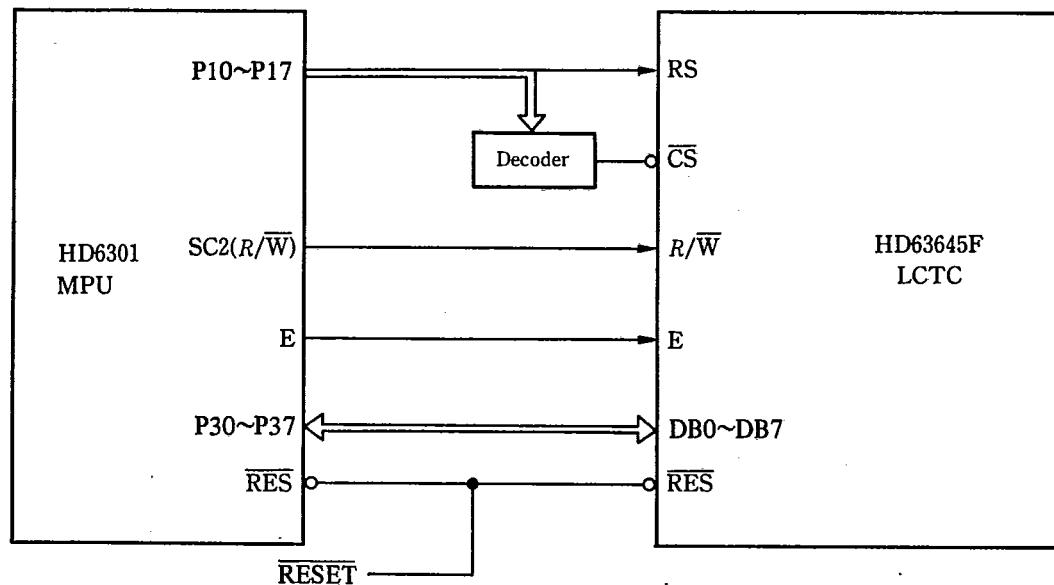
Note; HD6301 is set in mode 5. P10-P17 are used as output ports, and P30-P37 as data buses.
