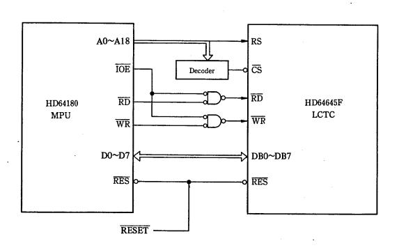
Note: Concerning 80 family MPU's, I/O space is separate from memory space in software. Thus the LCTC, a part of I/O, needs the ANDed signals of the interface signals and IOE. So IOE and RD, and IOE and WR should be ORed to satisfy t<sub>AS</sub>, the timing of CS, RD, and WR.
